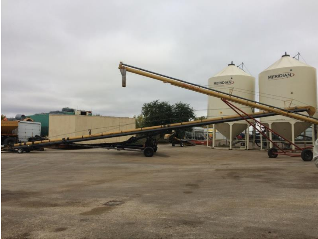
Photo 3-9: Hydraulic augers used to transfer raw seed to the seed storage bins.
