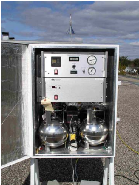
Figure 3. Volatile Organic Compound (VOC) Sampler Showing Summa Canisters
