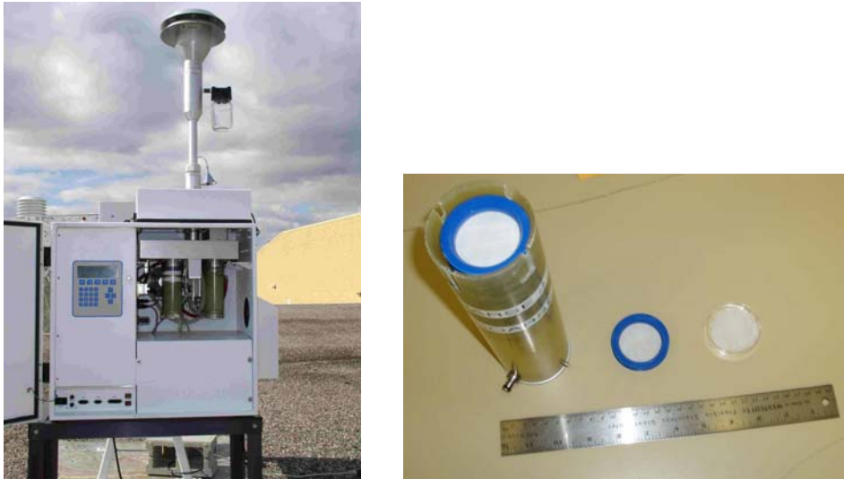
Figure 2. Dichotomous Partisol Sampler with Teflon Filters
