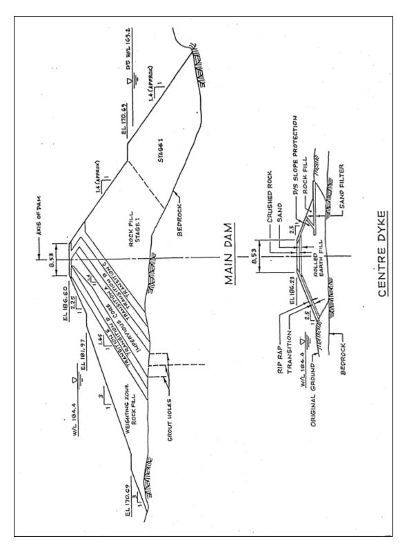
Figure 5 Kelsey GS Cross Section of Main Dam and Centre Dyke
