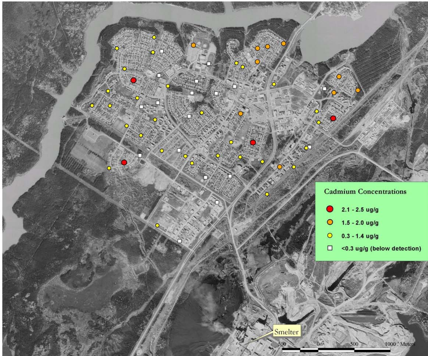
Figure 4. Aerial photograph of Thompson, MB, showing the ranges in Cd concentration in surface soil samples collected at 62 sample sites.
