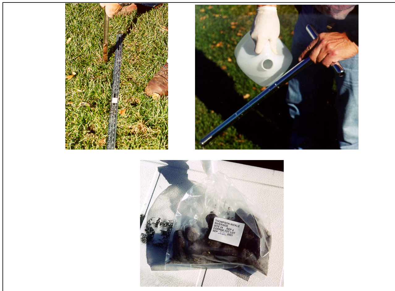
Figure 2. Photographs of soil sampling. Clockwise from upper left: (a) sampling using a small diameter soil coring tool; (b) rinsing equipment with distilled water between sample sites; (c) a replicate sample.
