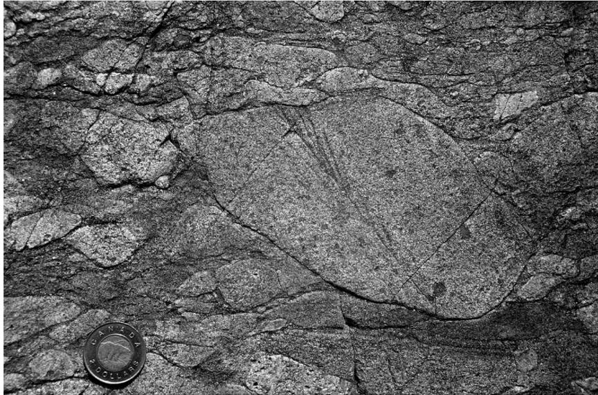
Figure GS-18-5: Intraformational, clast-supported conglomerate with psammite cobbles. Note crossbeds in the large clast in centre of photograph. Coin is 2.8 cm in diameter.
