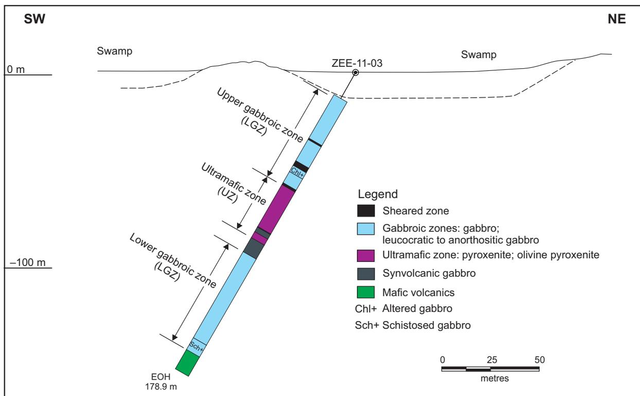
**Figure GS-7-3:** Schematic southwest–northeast geological cross-section of the Euclid Lake intrusion, illustrating the main geological units intersected in hole ZEE-11-03, drilled in 2011 by Mustang Minerals Corporation.
