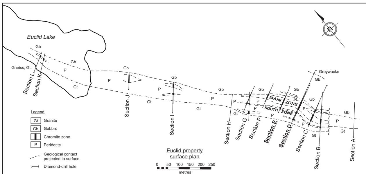
**Figure GS-7-2:** Surface plan of the Euclid Lake intrusion (after Robertson and Associates Ltd., 1981), presenting the projection of geological units as intersected in the 1942–1943 and 1952 drillholes. The locations of the 12 drill sections (A–L) compiled by Robertson and Associates Ltd. (1981) are also shown.
