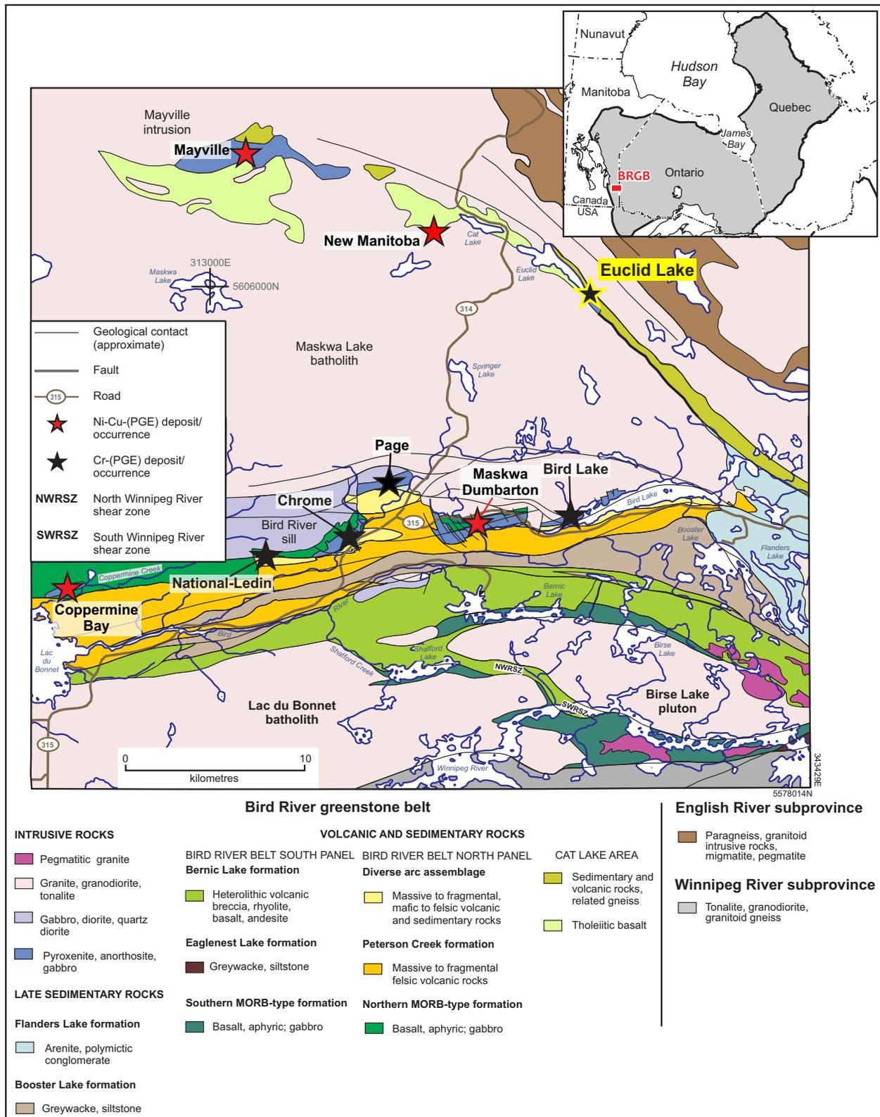
**Figure GS-7-1:** Simplified geology of the southern and northern arms of the Bird River greenstone belt, showing the location of the Euclid Lake intrusion and other significant mafic and ultramafic igneous bodies and their associated Ni-Cu-(PGE) and Cr-(PGE) deposits/occurrences (modified from Bailes et al., 2003; Gilbert et al., 2008). Abbreviations: BRGB, Bird River greenstone belt; MORB, mid-ocean-ridge basalt.
