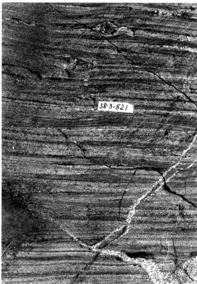
Figure GS-9-15: Layered amphibolite derived from pillow flow.
