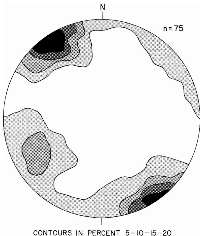
Figure GS-21-5: Lower hemisphere equal-area projection of pebble orientations in Inwood till. (25 pebbles were measured at each of sites 5, 20 and 26).
