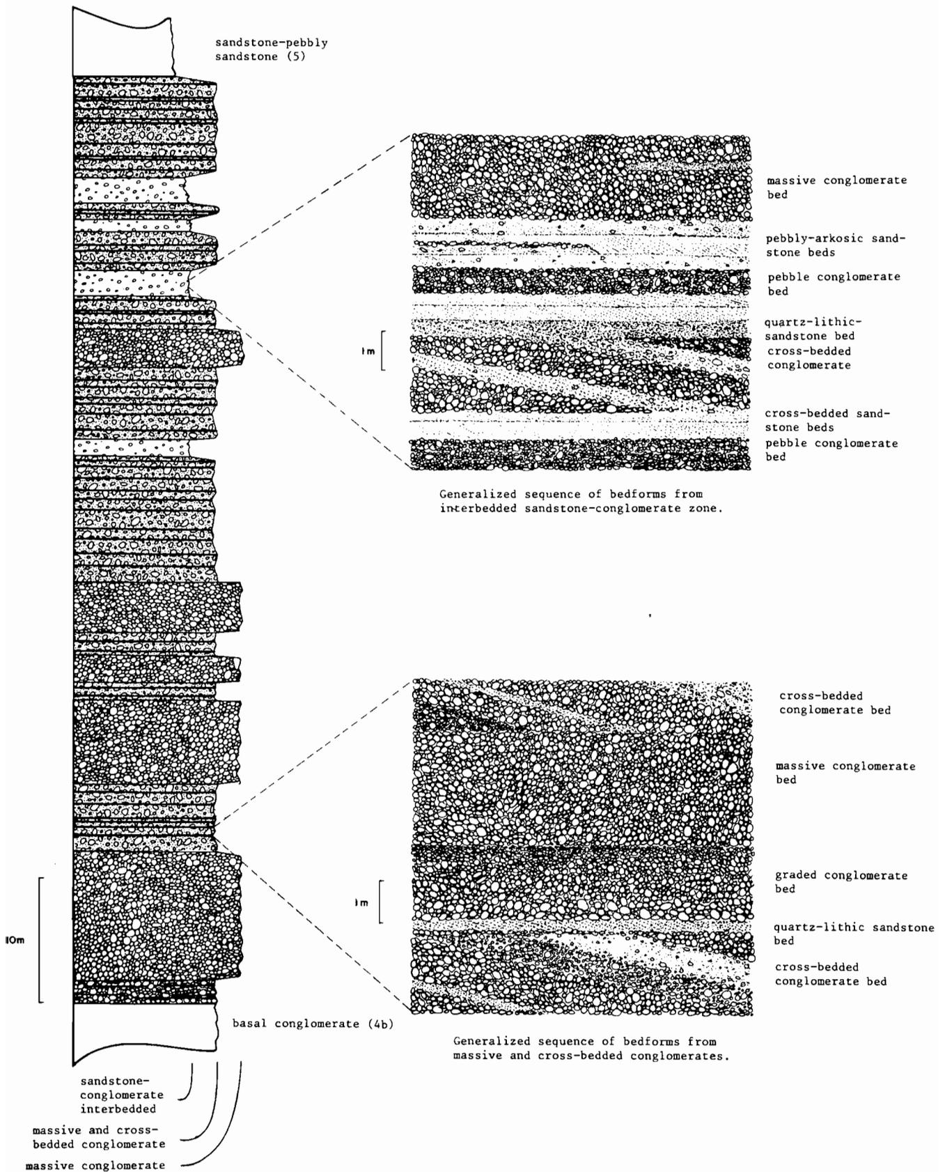
Figure GS-7-9: Stratigraphic section of conglomerate (4) - Pipestone Lake area - showing major bedforms.
