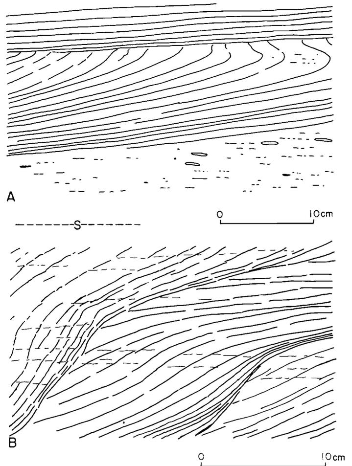
Figure GS-4-6: Two deformation fields of cross-bedding: (A) - from the limb of a major fold where bottomsets are close to the plane of flattening (S); (B) - from the hinge area of a major fold where foresets are close to the plane of flattening.
