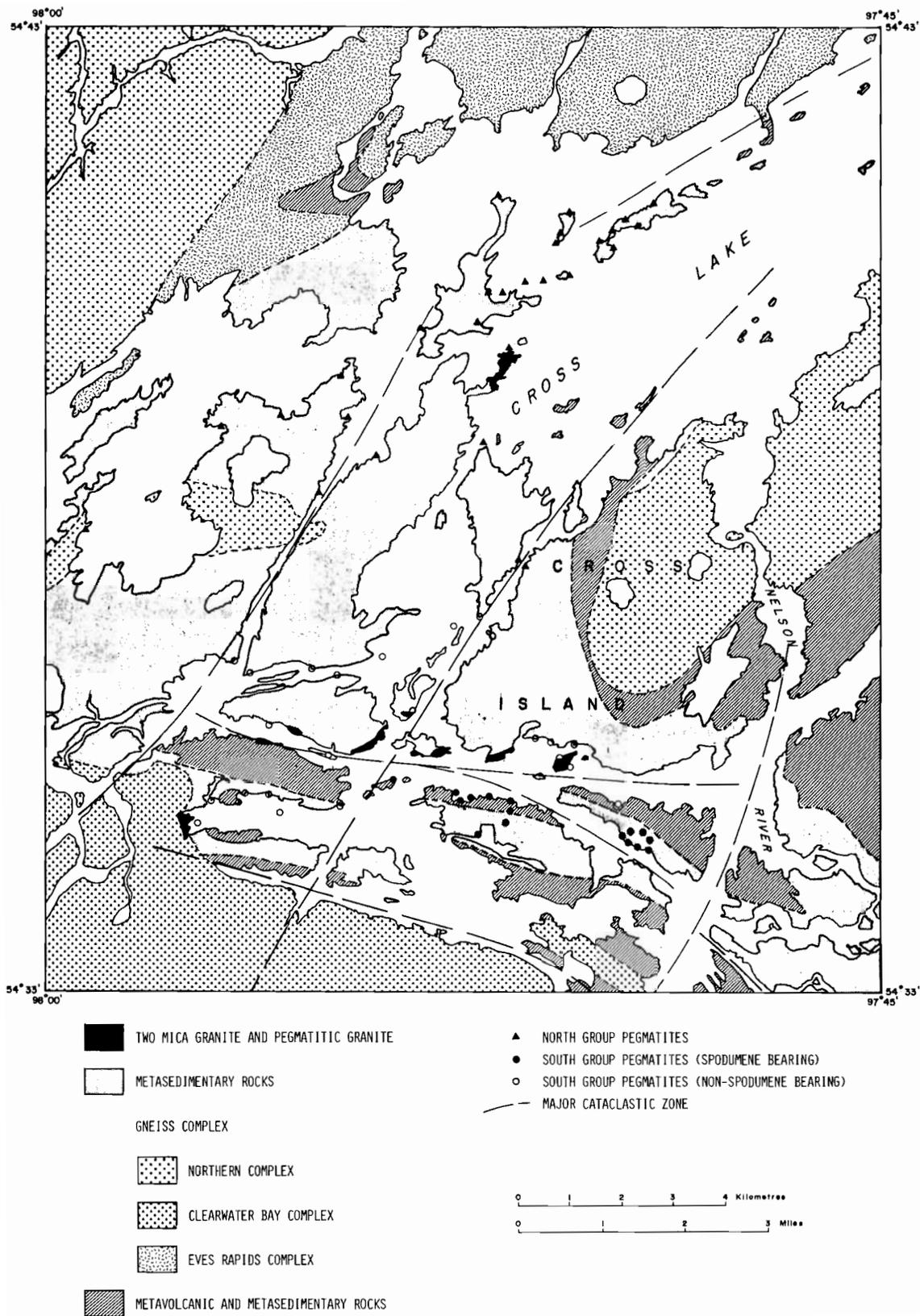
Figure GS-8-1: Simplified geological map of the Cross Lake area showing major structural features and the distribution of pegmatite dykes.
