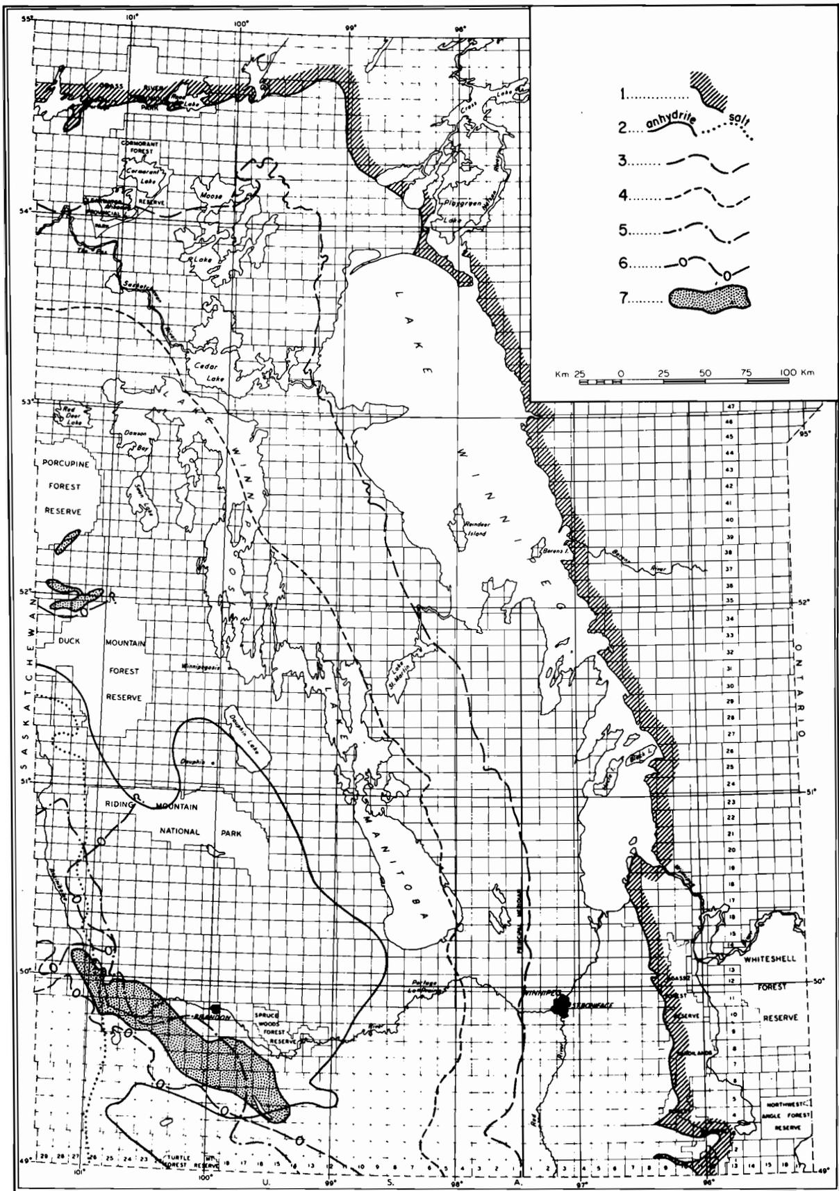
Figure GS-23-4: Sketch map showing eastern limit of Prairie Evaporite and features of sub-Mesozoic unconformity in relation to occurrence of Ashville sand: 1) southwestern perimeter of Precambrian Shield, 2) edge of Prairie Evaporite (anhydrite/salt): 3) northeastern limit of Silurian strata: 4) northeastern limit of Devonian strata: 5) northeastern limit of Mississippian strata: 6) depositional edge of Ashville sand: 7) area of thick Ashville sand.
