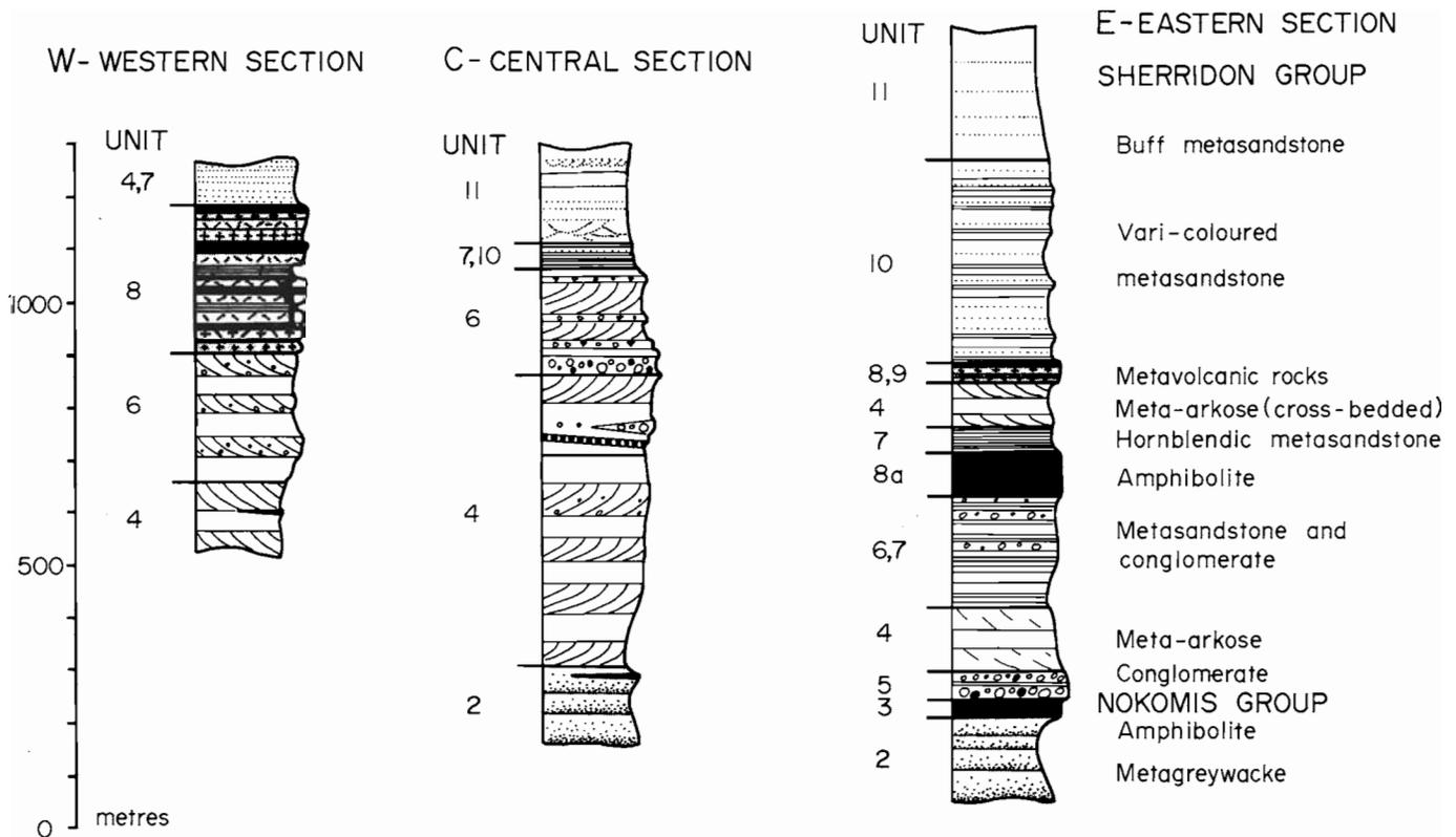
Figure GS-4-3: Preliminary stratigraphic cross sections based on a structural interpretation given in the text. Section lines are shown on Figure GS-4-2.
