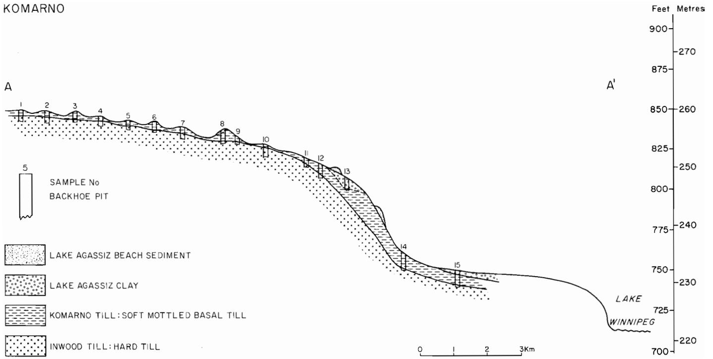
Figure GS-21-3: Stratigraphic cross-section of the surficial deposits in the Komarno area.
