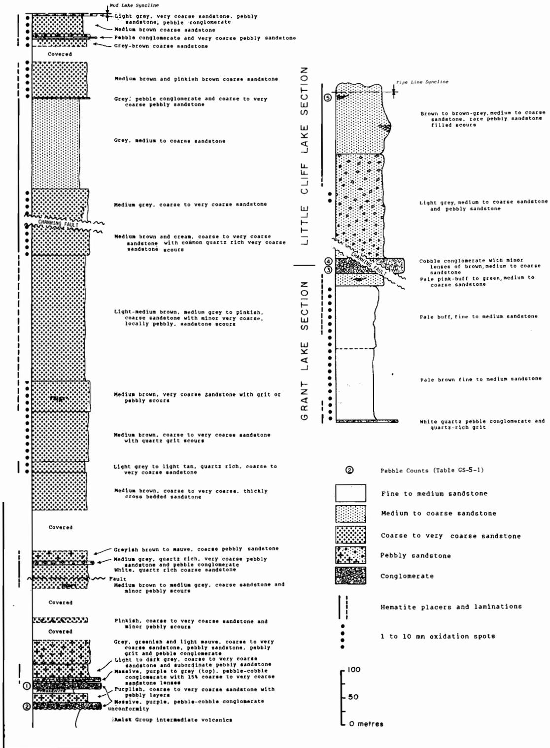
Figure GS-S-4: Measured section through the Missi Group in the south and east part of the Flin Flon (structural) basin. All of the sandstones are trough crossbedded; individual units shown are characterized by different crossbed set thickness, sand size, colour, quartz content, and the number, distribution and size of contained pebbles.
