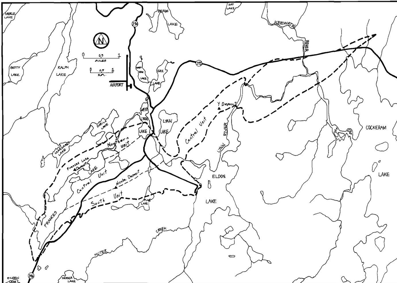
Figure GS-14-5: Preliminary breakdown of the stratigraphy of the Lynn Lake Rhyolitic Complex and the location of massive sulphide deposits contained in the complex.
