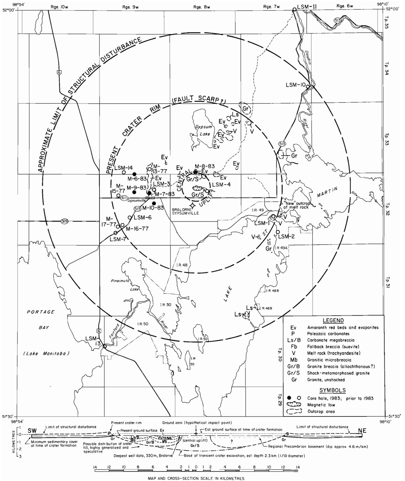
Figure GS-22-2: Geology and core hole locations, Lake St. Martin area, with true-scale structural cross-section.
