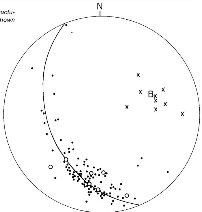
Figure GS-4-4: Equal-area stereogram of poles to bedding (dots) from the area of detailed mapping. Also shown are poles to axial planes of late minor folds (x) and fold axes (x). Note the great-circle distribution (solid line with pole B) indicating cylindrical folding. Upright and overturned beds follow this distribution and suggest sheath folding or refolding of early isoclinal folds.
