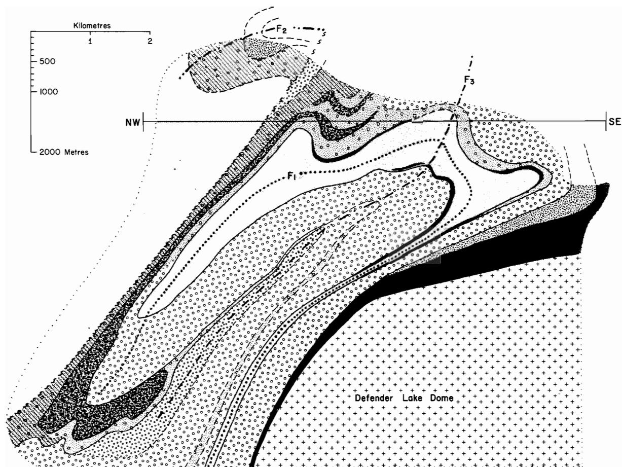
Figure GS-4-5: Structure section, projected down plunge (towards "8" in Figure GS-4-4) showing the early anticline ( $F_1$ ) refolded about a late antiform ( $F_3$ ) and the Defender Lake dome. The recumbent structure ( $F_2$ ?) at the top of the figure is schematic. The line of section and legend are shown in Figure GS-4-2.
