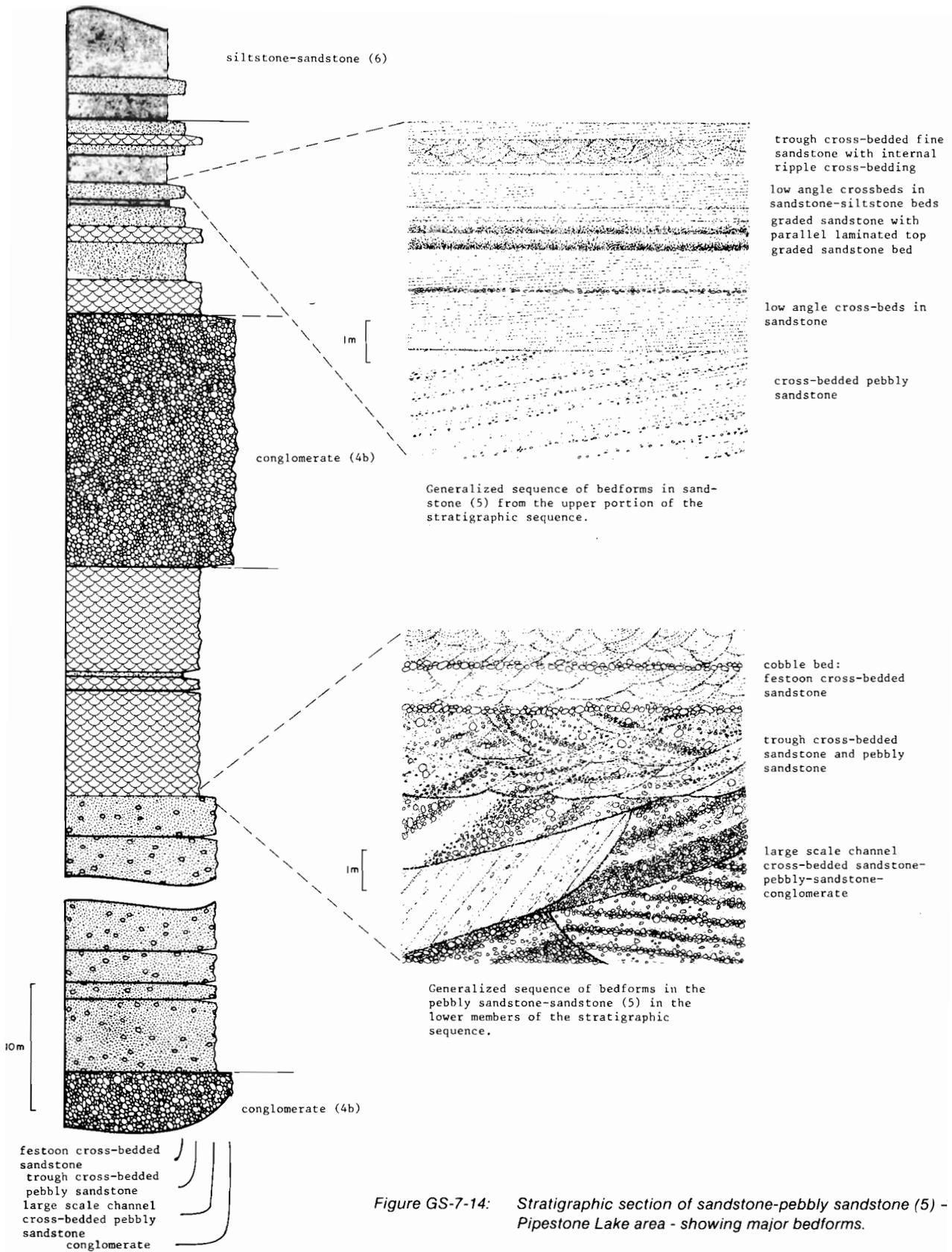
Figure GS-7-14: Stratigraphic section of sandstone-pebbly sandstone (5) - Pipestone Lake area - showing major bedforms.
