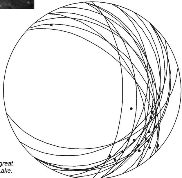
Figure GS-23-4: Lower hemisphere stereographic projections of  $S_1$  (great girdles) and  $L_1$  (dots) measured along the western shoreline of Edmund Lake.
