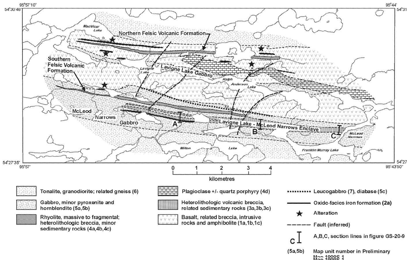
Figure GS-20-2: Simplified geological map of the southeast Max Lake area.
