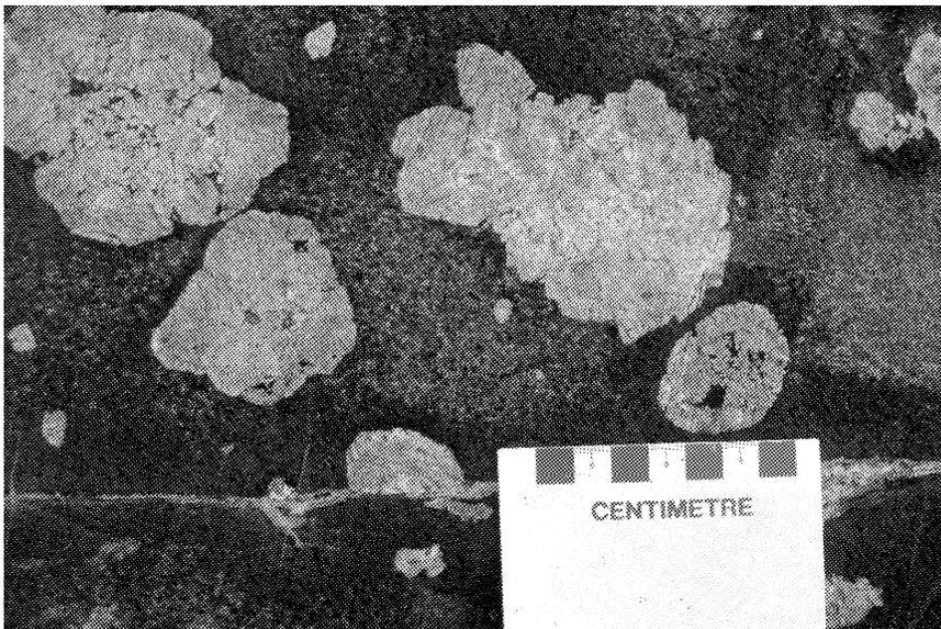
Figure GS-20-7: Pseudo-hexagonal plagioclase glomerocrysts in megaphyric gabbro (1c).
