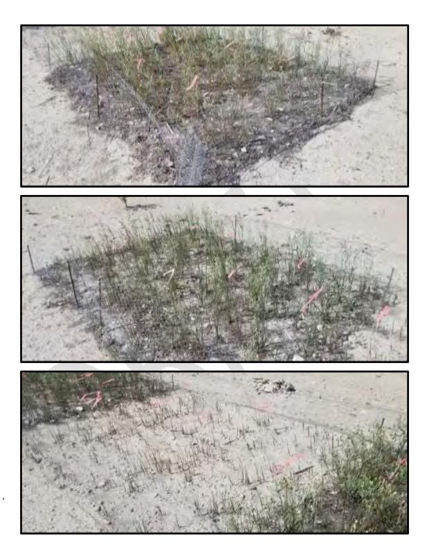
**Photo Array 4**: Site Inspection – August 8<sup>th</sup>, 2019 – Showing summer plant growth – 0.15 m organics depth (top), 0.075 m organics depth (middle), 0 m organics applied (bottom).
