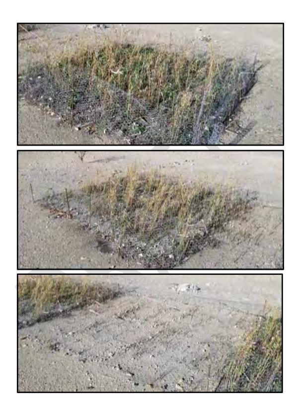
**Photo Array 6:** Site Inspection (September 23<sup>rd</sup>, 2019) – Showing late summer plant growth – 0.15 m organics depth (top), 0.075 m organics depth (middle), 0 m organics applied (bottom).
