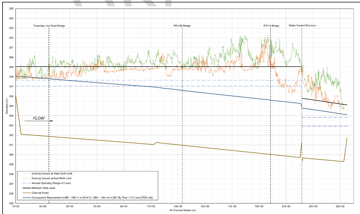
Figure 3: LMOC Water Surface Profile
