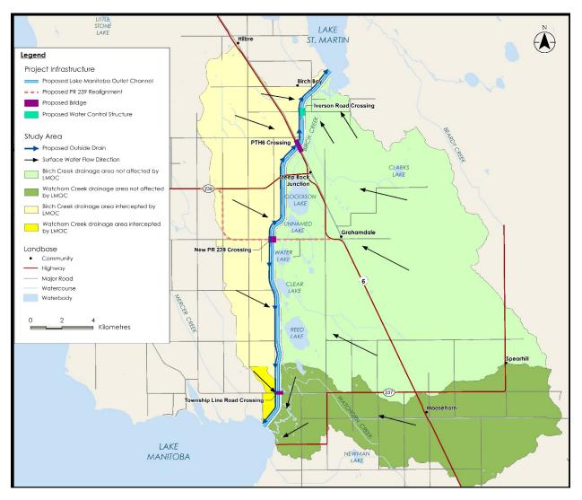
Figure 2: LMOC Outside Drain Arrangement
