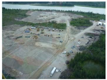
Photo 13: Borrow Pit Requiring Rehabilitation Post Construction
