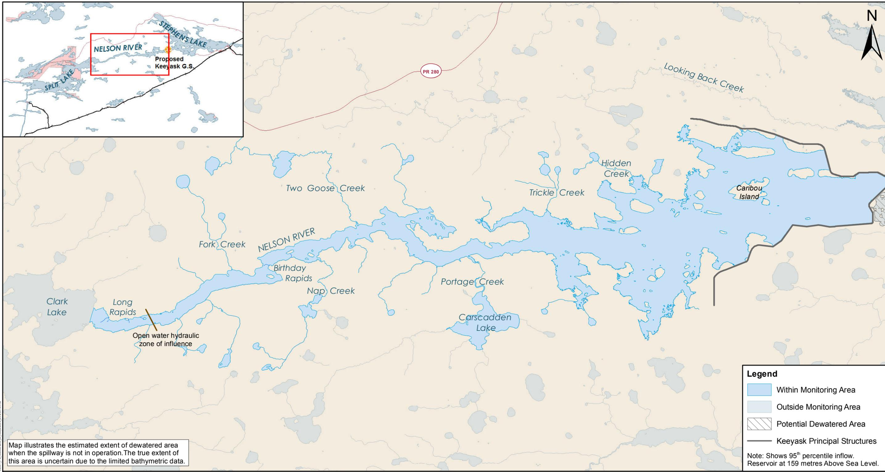
Map illustrates the estimated extent of dewatered area when the spillway is not in operation. The true extent of this area is uncertain due to the limited bathymetric data.
