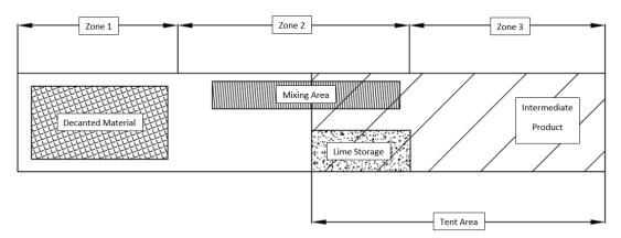
We have estimated that 200 T of intermediate product will be generated per day. Given the footprint of the processing area, the decanted material within the processing area will have a height of roughly 0.3 m and the mixing area height will be approximately 0.5 m high. A truck load of hydrated lime will need to be delivered to site every 1.5 days.
