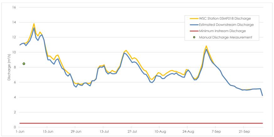
Figure 1: Average daily discharge upstream and downstream of diversion during irrigation period
