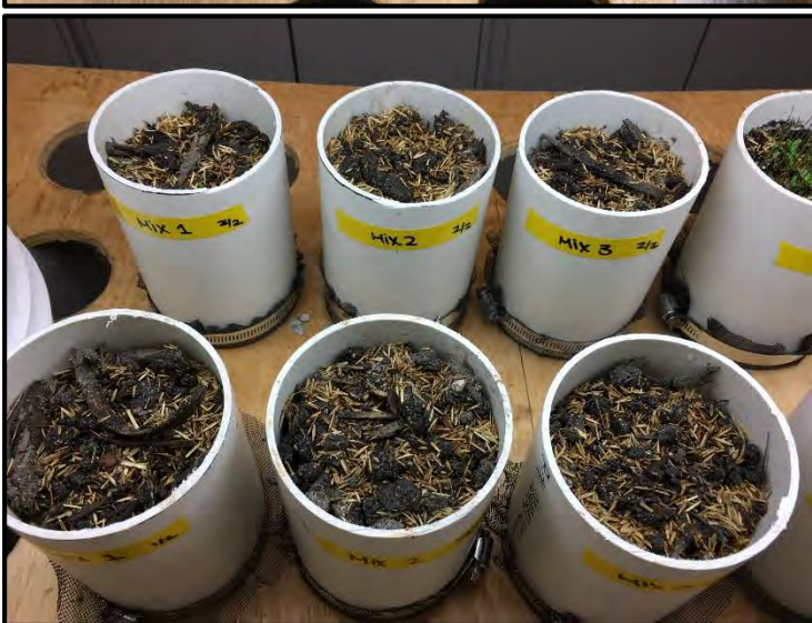
Photograph 9: Germination columns on Day 6 of the trial; germination is visible in the control columns but not in the test mix columns. (April 2, 2018)
