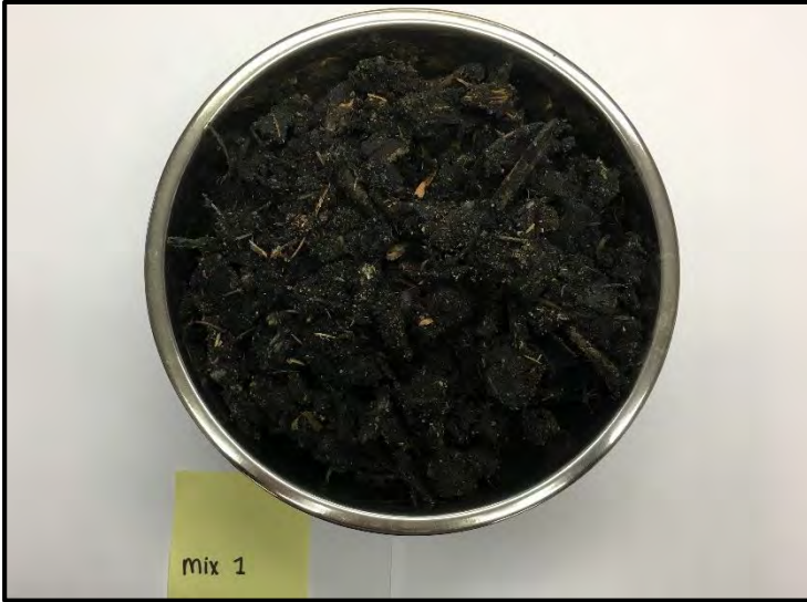
Photograph 4: Mix 1, blended at room temperature using the mechanical soil mixer. (March, 2018)
