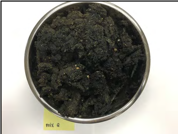
Photograph 5: Mix 2, blended at room temperature using the mechanical soil mixer. (March, 2018)
