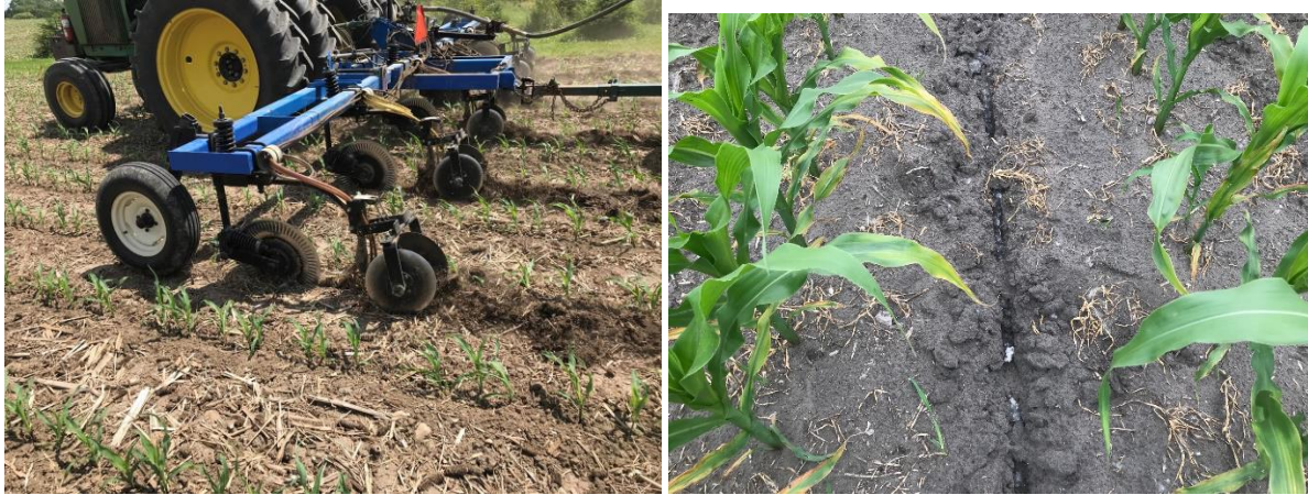
Figure 4-5. Ammonia slot sealing with closing disks (left) and leaf injury from unsealed slots (right).
