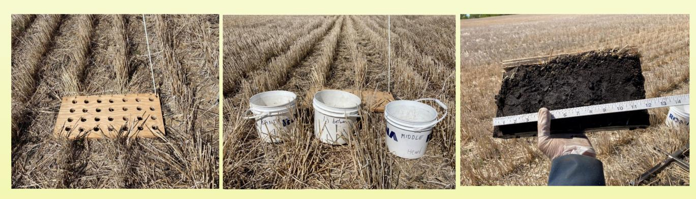
Figures 7-9. Soil sampling template (left), 3 pails (middle) and cross-section sample (right).
