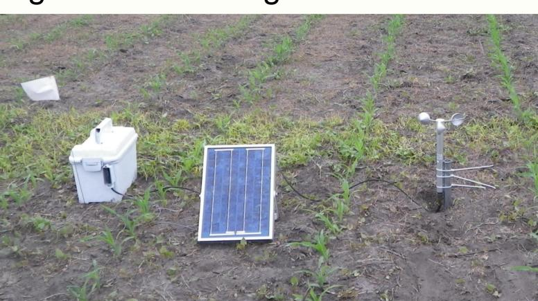
Figure 3. Solar powered data recorder and anemometer.
