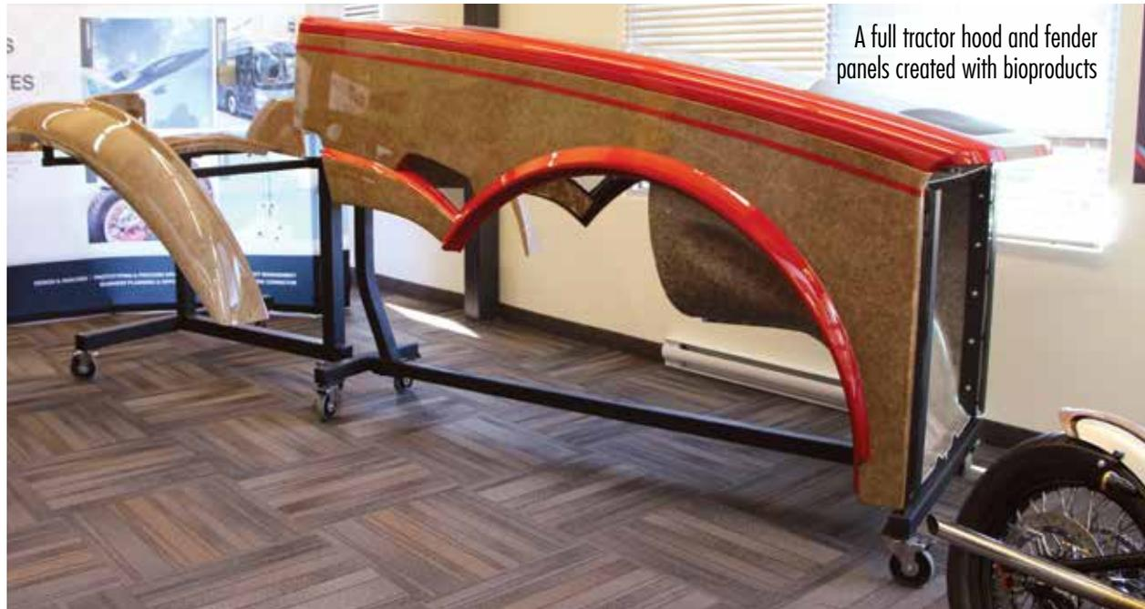
A full tractor hood and fender panels created with bioproducts
