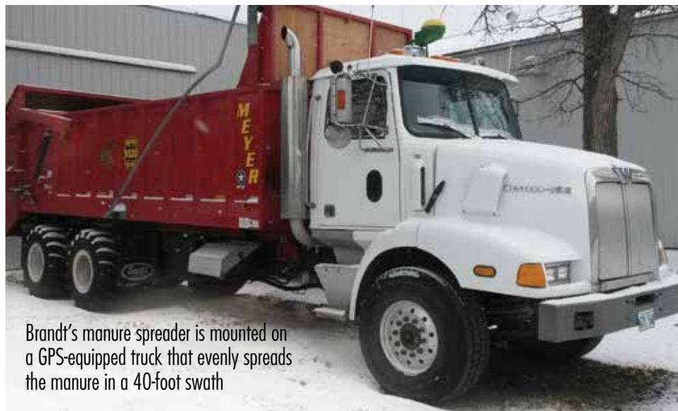
Brandt’s manure spreader is mounted on a GPS-equipped truck that evenly spreads the manure in a 40-foot swath
