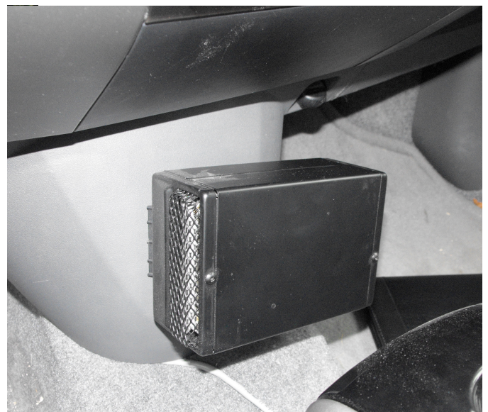
Customized winter front cover (left) and electric in-car warmer (right) implemented to address cold-weather cabin heating concerns
