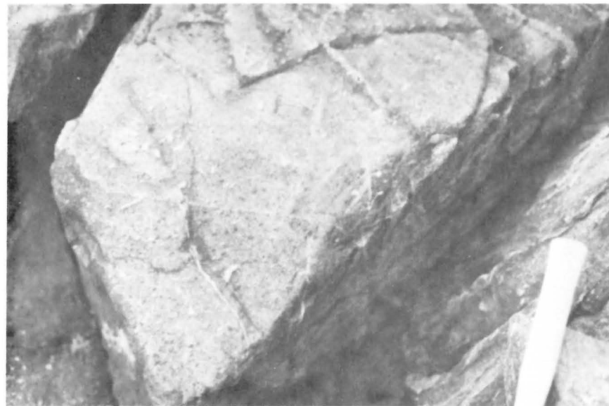
Figure GS-5-5: Hornblende (after pyroxene) and feldspar phenocrysts in weakly amygdaloidal andesite — Partridge Breast Lake
