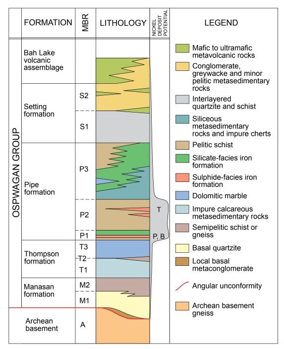
**Figure GS2018-1-4**: Schematic lithostratigraphic section of the Ospwagan group (modified from Bleeker, 1990). Abbreviations: B, stratigraphic location of the Birchtree ore body; MBR, member; P, stratigraphic location of the Pipe II ore body; T, stratigraphic location of the Thompson ore body.
