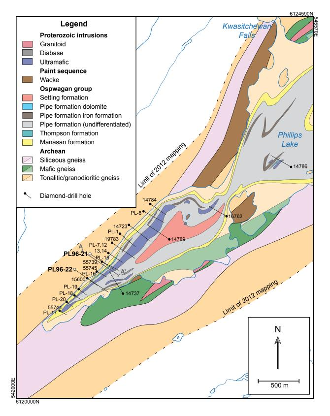
**Figure GS2018-1-3**: Composite geology of southern Phillips Lake, showing the locations of diamond-drillholes by Inco Ltd. (five-digit numbers) and Falconbridge Ltd. (beginning with 'PL'). The geology underlying the lake is from Macek et al. (2006) and the shoreline geology is from Couëslan (2016). The section in Figure GS2018-1-2 is along line A–A' (in grey)
