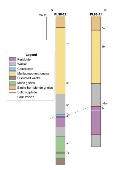
**Figure GS2018-1-5:** Schematic logs of drillcores PL96-21 and PL96-22 in the southern Phillips Lake area; see Figure GS2018-1-3 for drillhole locations. The approximate locations of images in Figures GS2018-1-6 and GS2018-1-7 are indicated along the right-hand side of each column.
