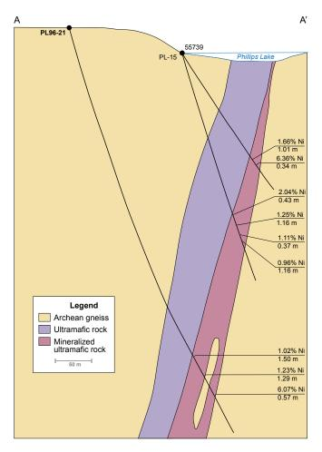
**Figure GS2018-1-2:** Cross-section A–A', looking north through Falconbridge Ltd. drillholes PL-15 and PL96-21, and Inco Ltd. drillhole 55739 (modified from Assessment File 94497). The locations of drillholes and section A–A' are shown in Figure GS2018-1-3.
