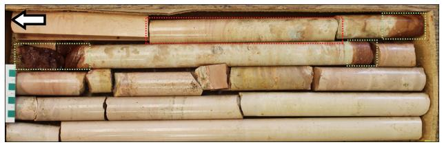
*Figure GS2018-12-5:* Photograph of core from drillhole Neepawa DDH No. 1 Prov. 15-29-14-14W1 from 458.70 to 461.80 m. Two red, argillaceous, crinoid-rich beds are outlined in green dashes, and the single stromatoporoidal bed is outlined in red. Arrow indicates up direction in core. Scale bar in centimetres.
