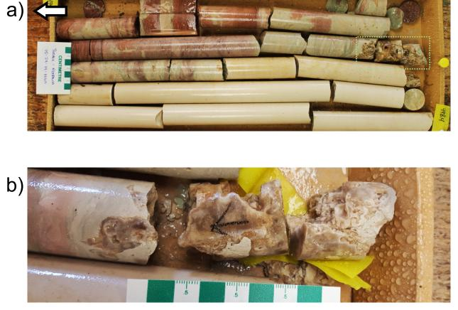
*Figure GS2018-12-4:* Diagenetic alteration of the East Arm Formation in drillcore from Neepawa DDH No. 1 Prov. 15-29-14-14W1: a) photograph of dolostone from 495.30 to 498.40 m, zone of alteration outlined in green dashes; b) photograph of diagenetic alteration from 496.53 to 496.65 m, scale bar in centimetres. Arrow indicates up direction in core.
