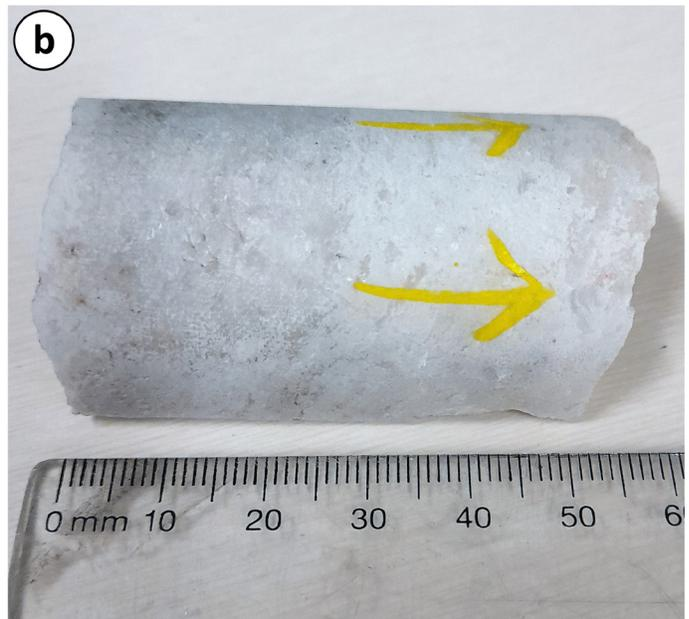
**Figure GS2021-2-3:** Drillcore samples showing **a)** large central apatite crystal (blue) with secondary metasomatic microcrystalline mica halo (green) within pale grey SQUI (sample CB18.08.21, 91-10, B5C3, 173.9–174.4 ft); and **b)** classic SQUI intergrowth textures after petalite (sample CB12.08.21, 94-12, B3C2, 95–95.2 ft).
