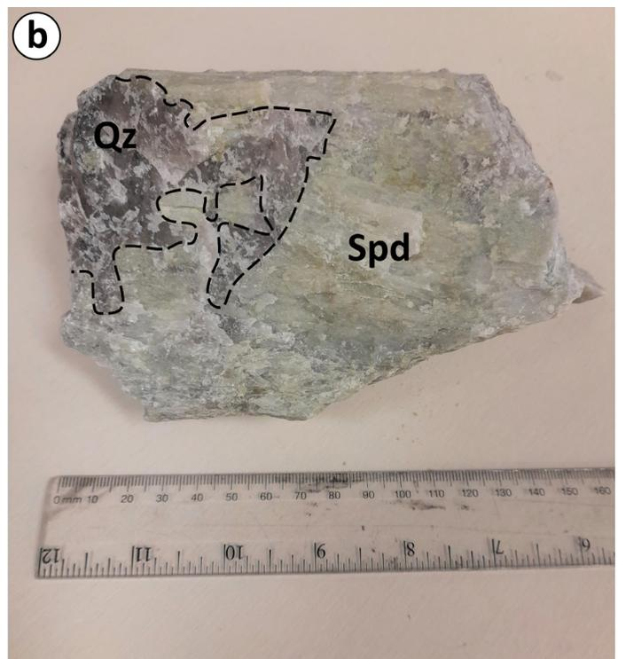
**Figure GS2021-2-4:** Underground images and samples showing **a)** large in-place SQUI (spodumene and quartz intergrowth) crystal showing characteristic replacement textures (highlighted with dashed line; hand for scale); and **b)** sample of green spodumene (Spd) and smoky quartz (Qz) from the Li-rich zone.
