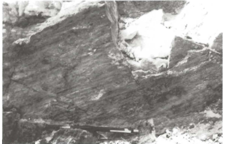
Figure GS-2-7: Slickenside striae in the main fault. The faulted rock is the main (quartz) vein described in the text. Looking west.
