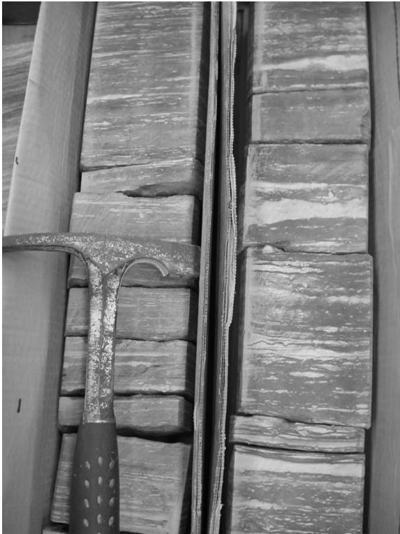
**Figure 11 - Bioturbated and interbedded sandstone and siltstone of a widespread marker unit at the base of unit C (centred around approximately 1942.0m) in the 15-10-6-19W2 well in the Ceylon Pool.**
