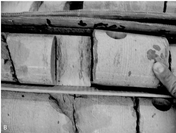
**Figure 8 - A) Silty, argillaceous, very fine-grained quartz sandstone reservoir rock of units A1 and B between arrows (i.e. 1589.0-1594.4m) in the 7-6-8-8W2 well; note that oil staining is a pale light brown and almost invisible to the naked eye. B) Close-up of unit A1 reservoir rock; note the presence of large pyrite nodules and pyrite-rich interlamination.**
