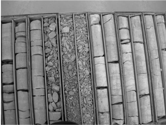
**Figure 13 - Variably coloured, oxidized Upper and Middle Bakken members overlain by tan to whitish limestones of the Souris Valley between approximately 490.5-499.0m in a well at 14-16-18-30W1.**
