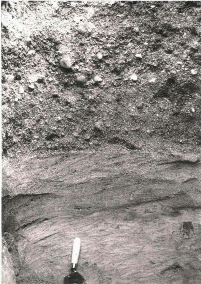
FIGURE 5: Sandy pebble gravel overlying sand in central portion of outwash plan; NE 28-22-29W. Trowel is 28 cm long.
