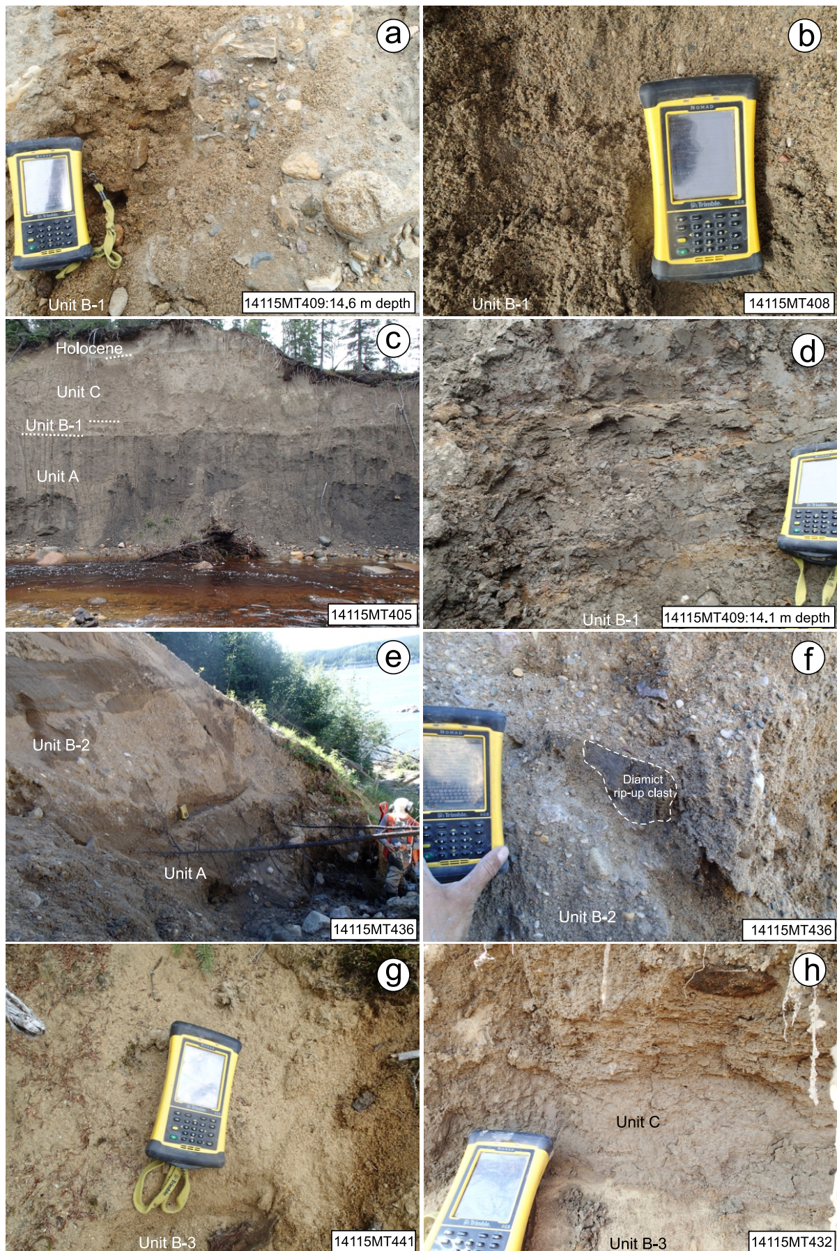
Figure 13: Photographic examples of Unit B clay, sand and gravel; including lithofacies B-1 (a–d), B-2 (e, f) and B-3 (g, h) from six different sections along the Churchill River. The label refers to the site number.
