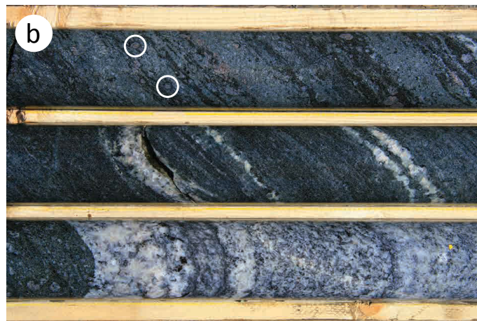
Figure 4: Drillcore images of hornblende gneiss and calcsilicate: a) hornblende gneiss grading into plagioclase amphibolite (top two rows), circles indicate plagioclase pseudomorphs after garnet (HZ-19-1, 76.4 m); b) calcsilicate interlayered with hornblende gneiss (top two rows), circles indicate garnet porphyroblasts (HZ-19-1, 221.65 m); c) discordant zone of calcsilicate (top row, outline in white) hosted in hornblende gneiss (the trace of the regional rock fabric/layering is outlined in yellow), the hornblende gneiss is intruded by pegmatitic granite that is locally hornblende- and titanite-bearing (bottom row; HZ-19-1, 81.55 m). Drillcore is NQ with a diameter of 47.5 mm.
