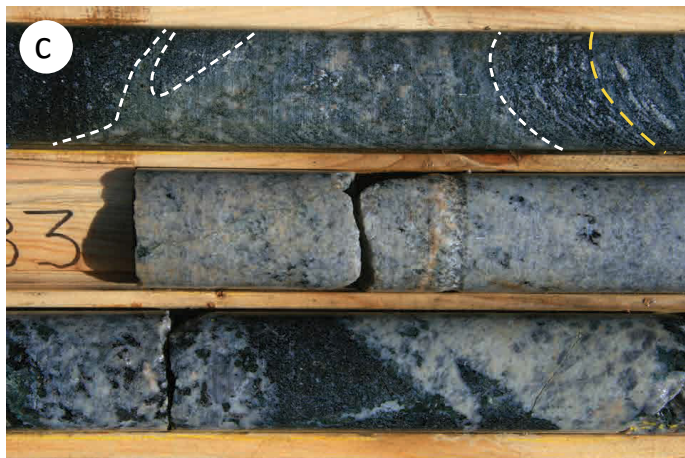
Figure 4: Drillcore images of hornblende gneiss and calcsilicate: a) hornblende gneiss grading into plagioclase amphibolite (top two rows), circles indicate plagioclase pseudomorphs after garnet (HZ-19-1, 76.4 m); b) calcsilicate interlayered with hornblende gneiss (top two rows), circles indicate garnet porphyroblasts (HZ-19-1, 221.65 m); c) discordant zone of calcsilicate (top row, outline in white) hosted in hornblende gneiss (the trace of the regional rock fabric/layering is outlined in yellow), the hornblende gneiss is intruded by pegmatitic granite that is locally hornblende- and titanite-bearing (bottom row; HZ-19-1, 81.55 m). Drillcore is NQ with a diameter of 47.5 mm.
