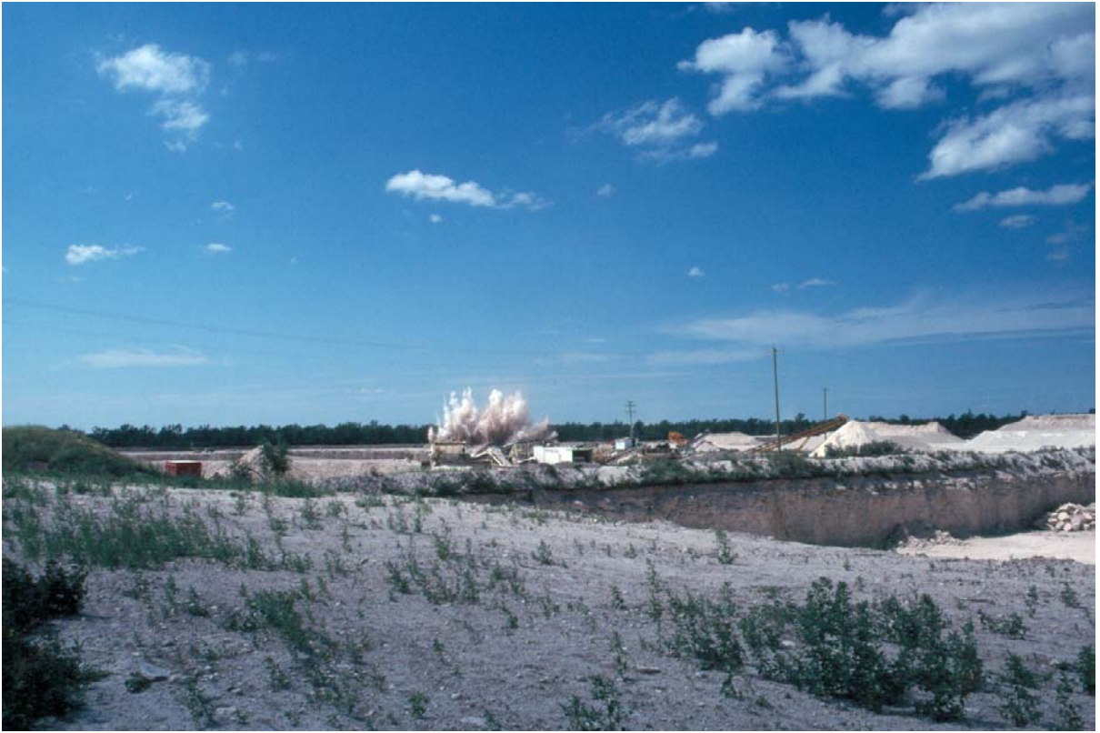
B.A. North 01 - 1995-07-13, B.A. Quarry North. Gunton Member of the Stony Mountain Formation. Blasting of bedrock.
