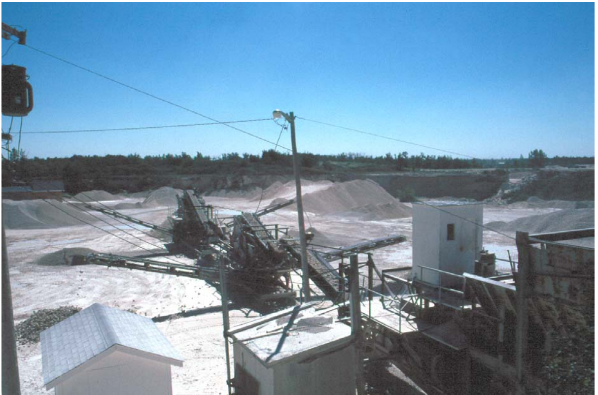
Standard 03 - 1995-07-12, Crusher and sorter at Standard Quarry South.
