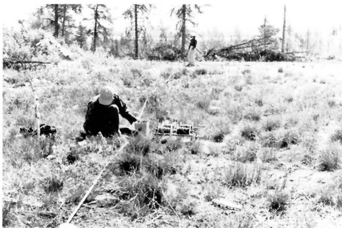
PLATE 19A: Equipment used in resistivity profile work: meter, coils, 30 m tape and electrodes spaced according to the Wenner configuration. Location: eastern margin of Leaf Rapids esker.
