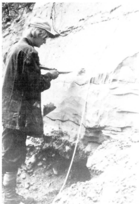
PLATE 10A: Unit 3 glaciofluvial gravel exposed at base of thick laminated silt and clay section (Unit 4).
