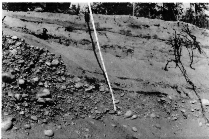
PLATE 8A: Parallel laminated and accretionary foreshore sand overlying coarse glaciofluvial sediments. Note wave-cut notch at contact at B49W. Measured section 1.0 m.
