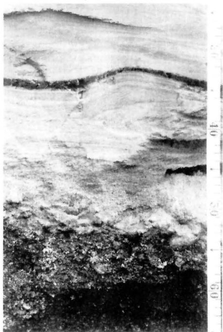
PLATE 13A: Detail of contact between silt and glaciofluvial sand and gravel towards base of section 66-67 north. Paleoflow direction in medium-fine ripple drift cross-stratified sand indicates current from right to left in photo (from northeast to southwest). Scale in centimetres.
