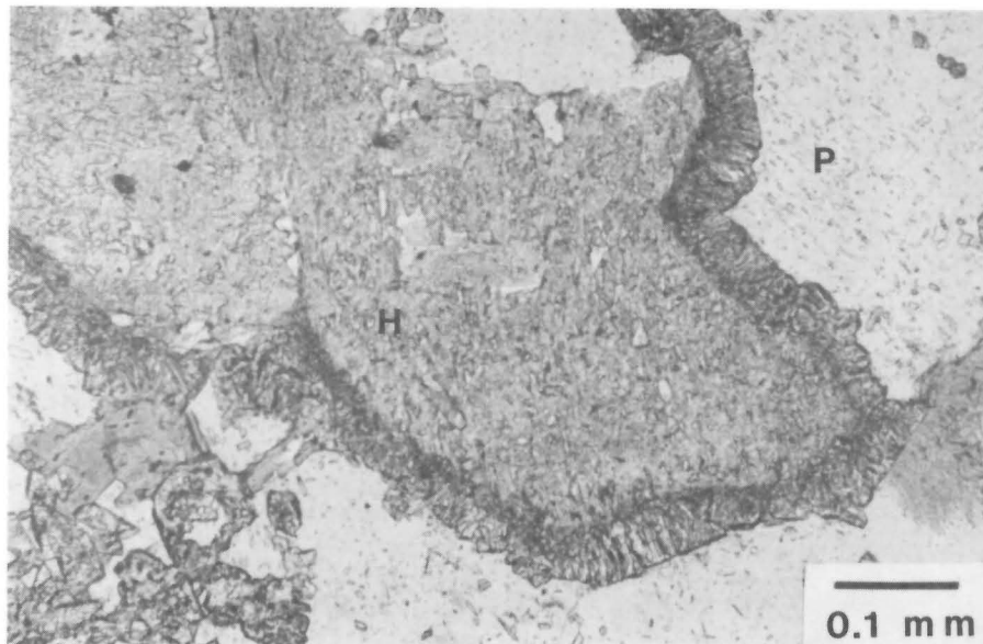
FIGURE 50: Photomicrograph (plain light) of relict M_1 granoblastic textures in M_3 metamorphism. Mafic aggregates—dominantly M_2 hornblende (H)—in contact with plagioclase (P) have a corona of epidote and quartz developed during M_3 metamorphism.
