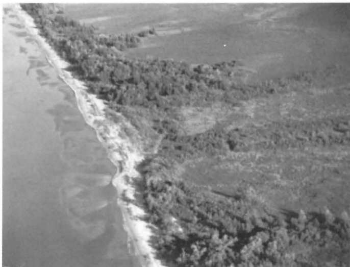
Figure 29: 'Closed' washover at Site 2, near the mouth of West Channel. Note the absence of trees at the site of the washover and the southward extent of this and older washovers into the marsh as defined by rows of shrubs and trees. Notice the extensive longshore bars along the shore.
