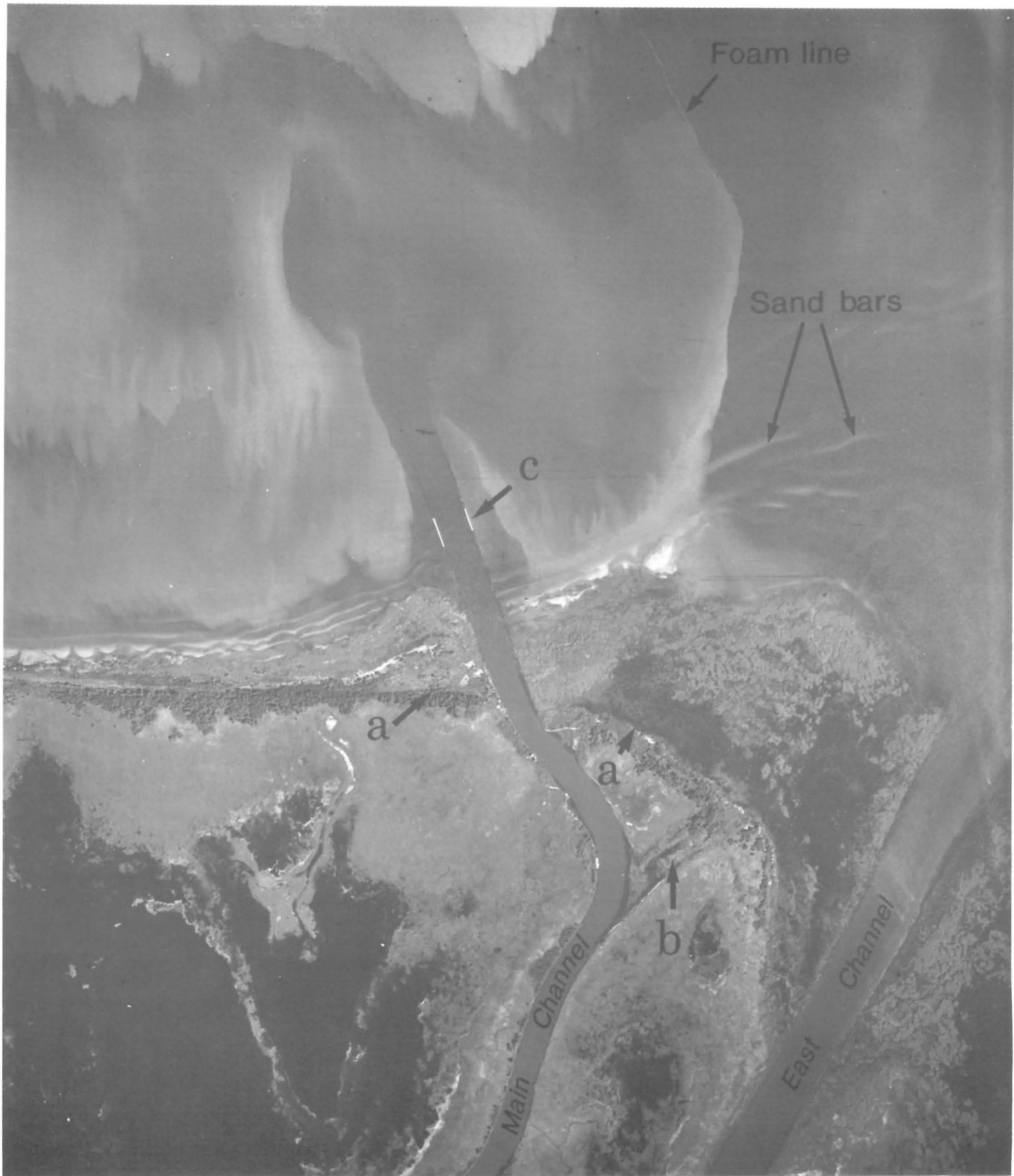
Figure 53: Airphoto from 1946 showing the mouth of Main Channel. The pre-1900 shoreline is marked (a), the pre-1900 channel (b) and the breakwater (c). Note the foam line, longshore bars and differences in the water transparency.
