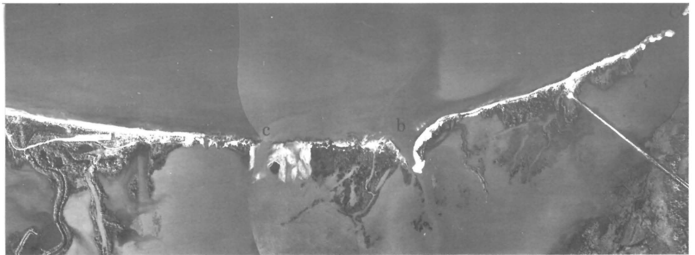
Figure 49: Airphotos of the bay-mouth-bar at Beaconia Lake showing the changes in the inlets between (A) 1946, (B) 1966, and (C) 1971. The inlets are labelled (a), (b) and (c).
