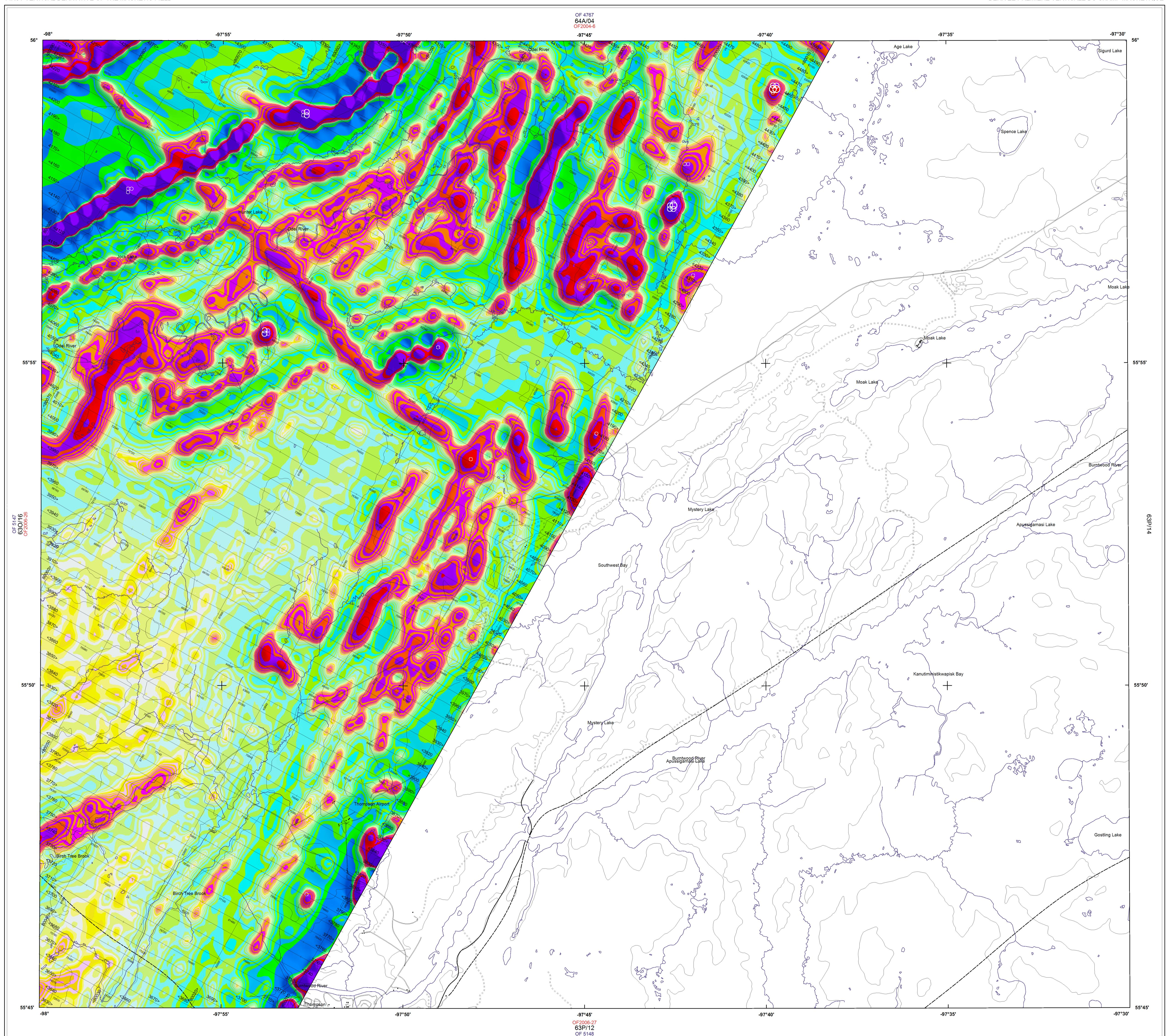
This map was compiled from data obtained as a result of an aeromagnetic survey carried out by Goldak Airborne Surveys using a Piper Navajo (registration C-GJBB) aircraft. A magnetometer, mounted on a beam, cesium vapour magnetometer was mounted in the tail boom of the survey aircraft.
