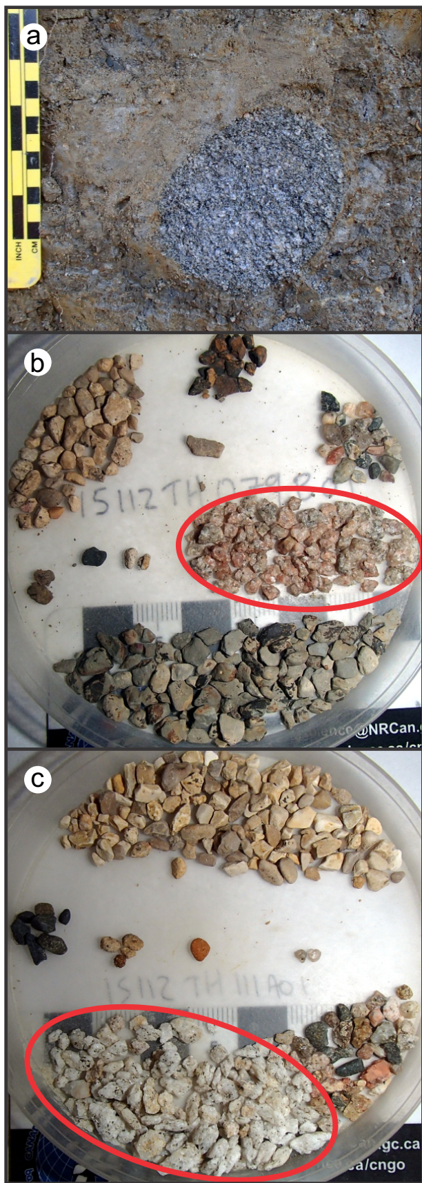
Figure 7: Evidence of chemical weathering observed in till-clast counts and within till exposures observed in the field: a) chemically weathered granite cobble in till at station 15112TH156 which disintegrates into sand-size fragments when moved; b) micaceous tonalite clasts highlighted by the red ellipse in sample 15112TH111A01; and c) quartz syenite clasts highlighted by the red ellipse in sample 15112TH079B01.
