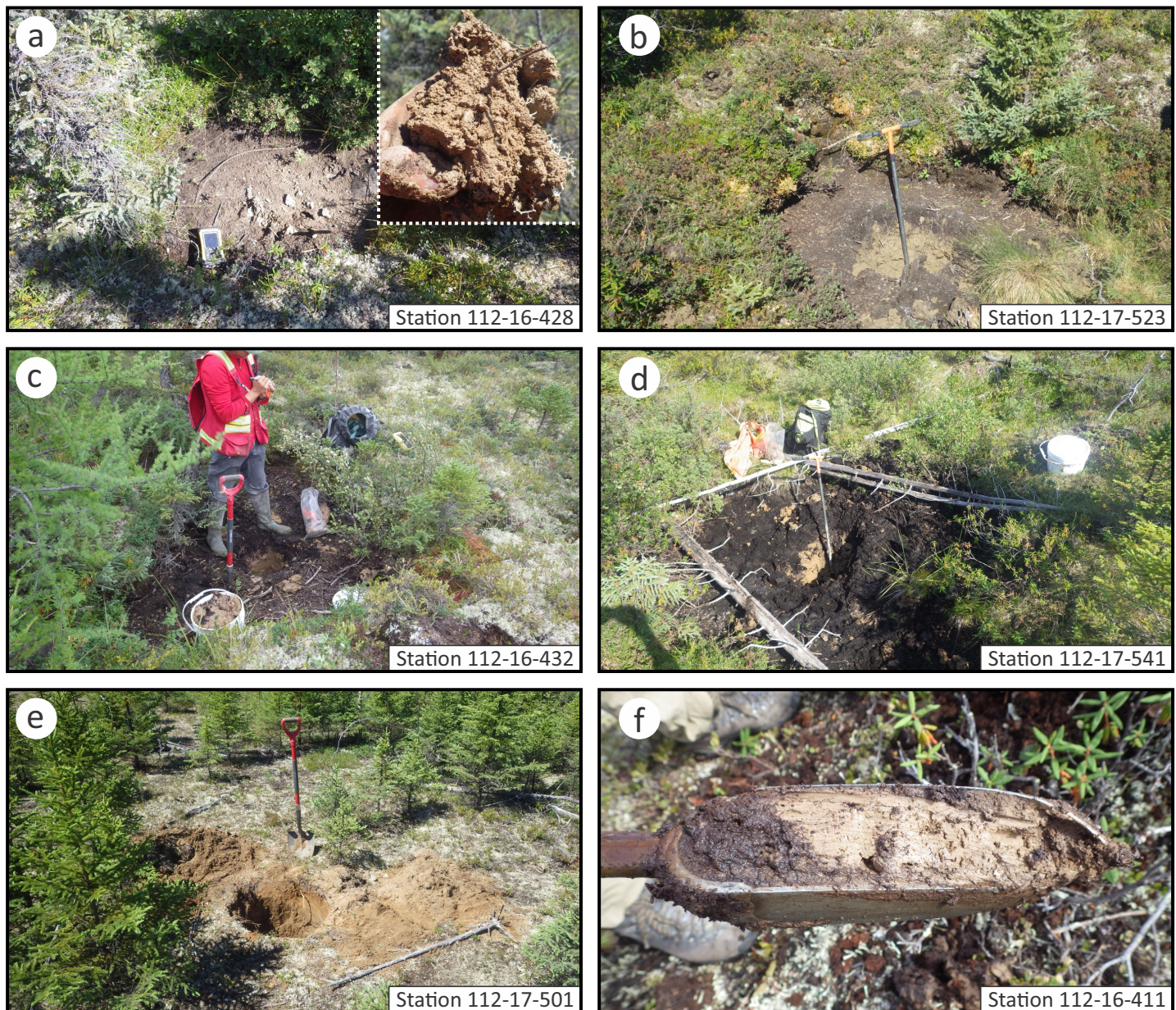
Figure 6: Example of surface till sampling sites in the Kaskattama highland area: a–d) example of mudboils that were used to sample unweathered till; e) example of a hand-dug pit in a region with no mudboils that was used to sample C-horizon till at depth; f) example of C-horizon till sample that was sampled at depth underlying organic material using the assistance of a dutch auger.
