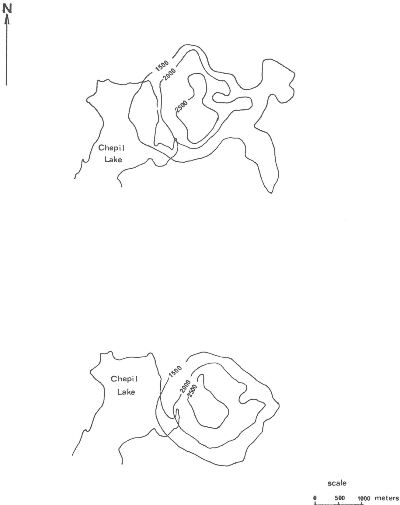
FIGURE 4.13 Magnetic anomalies near Chepil Lake. The top diagram is the anomaly field, the bottom diagram is the model field, the values are the magnetic field in nT with a subtraction of 60 000 nT.
