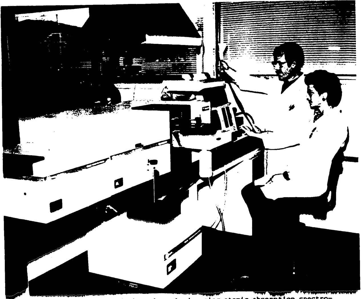
Frontispiece: Rock and mineral analysis using atomic absorption spectrophotometry, Logan Avenue Laboratory, Winnipeg.
