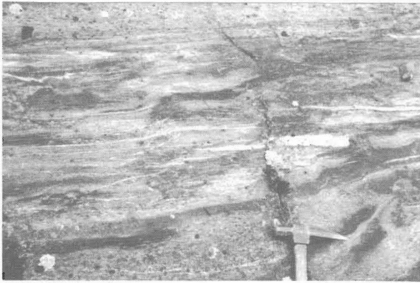
Fig. 3: Deformed metabasalt (1b) with hornblende-rich pillow selvages (thin dark layers), Moody Lake.
