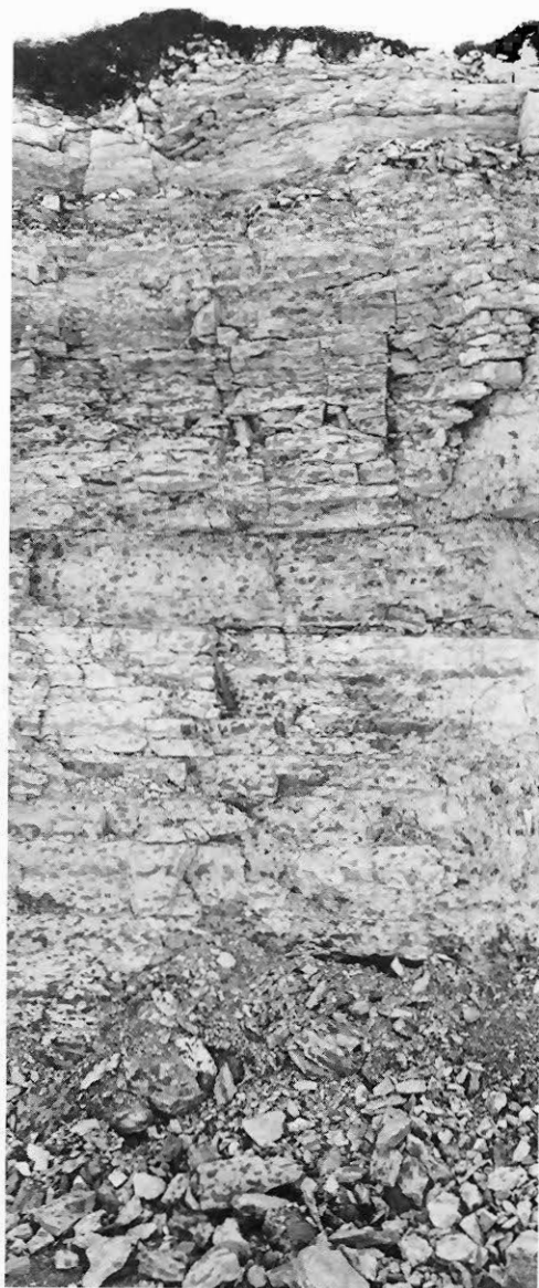
PLATE 6. Location of measured section, south wall of Department of Highways quarry; note variation in mottling. The lighter areas have a higher MgO content than the darker mottles.
