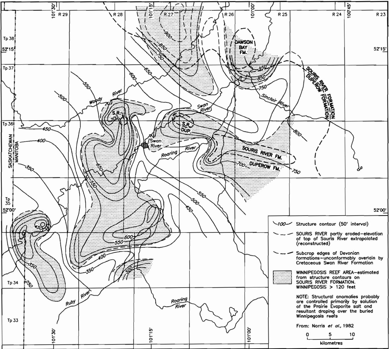
Figure 22: Detailed structure contour map, Souris River Formation, Swan River area (modified after Norford *et al.*, 1982).
