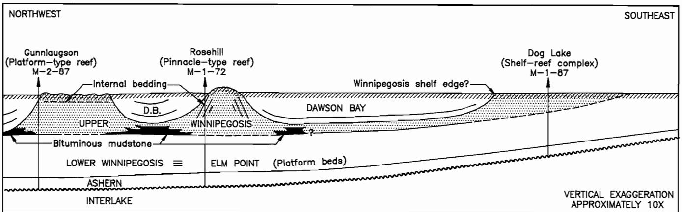
Figure 31: Diagrammatic cross section, Winnipegosis Formation reefs, The Narrows area.
