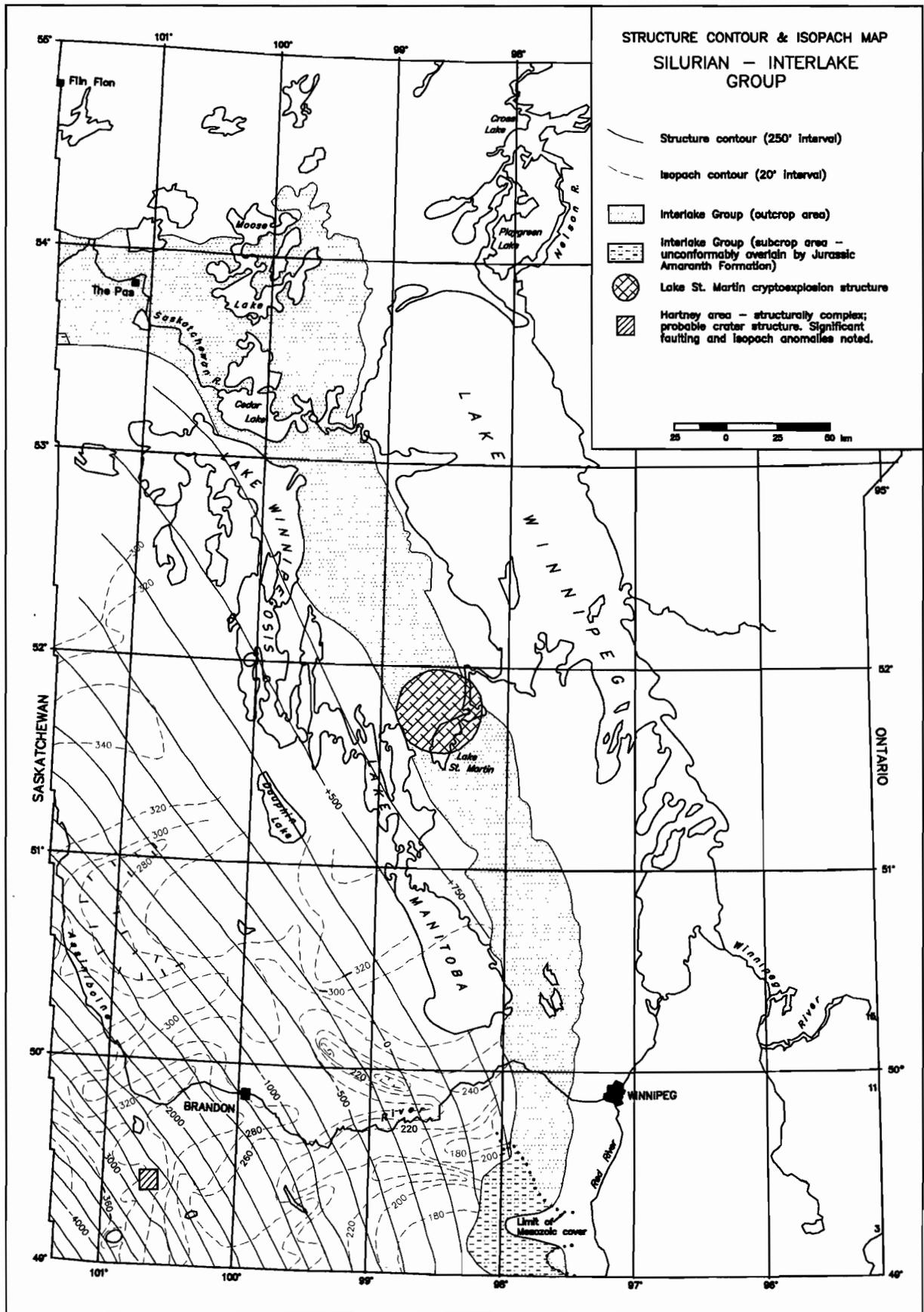
Figure 10: Interlake Group structure contour and isopach map (modified from Martiniuk, 1992).
