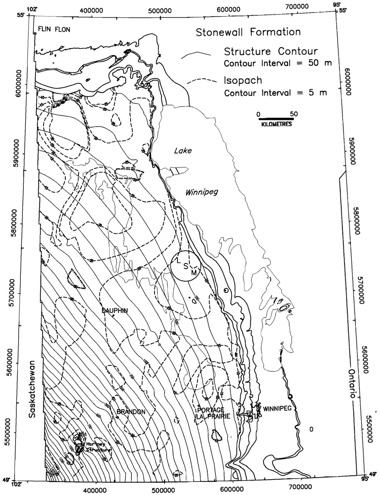
Figure 8: Stonewall Formation structure contour and isopach map.
