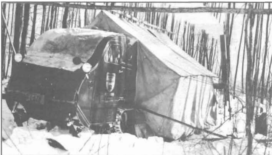
Heating Bombardier so that it will start in the morning
