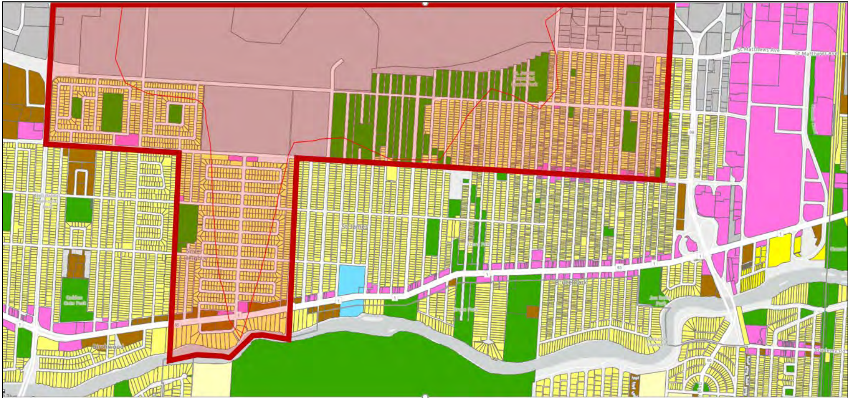
Figure 5-11 – Sample Boundary Selection Exercise – Revised Area I Boundary Interpreted from Ultimate-Term 35 NEF Contour
