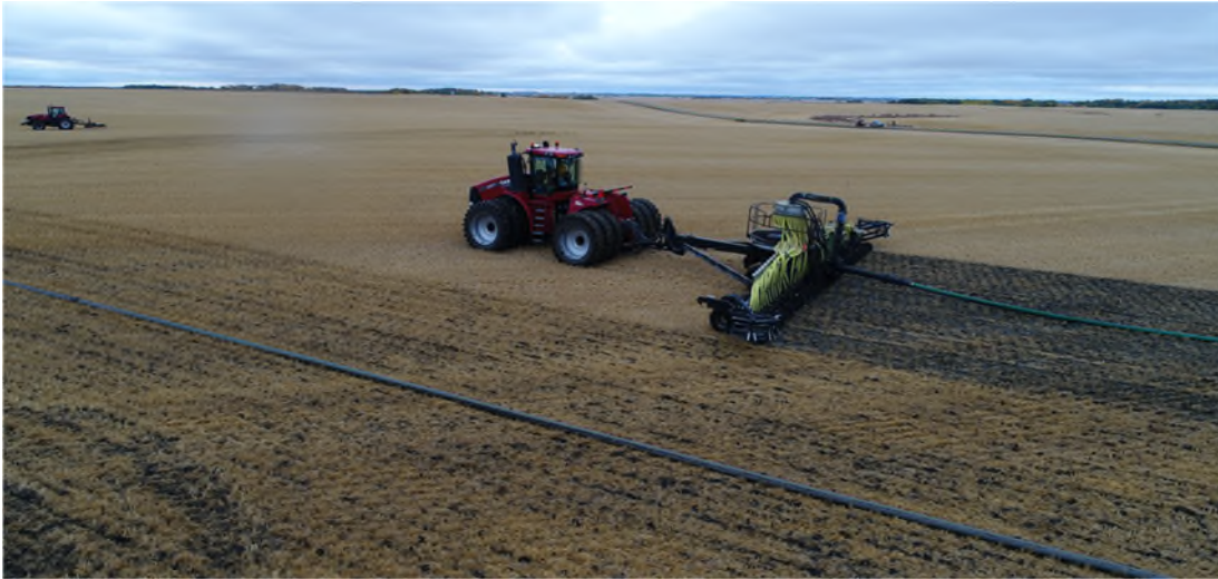
8" Forcemain Connecting to Manure Applicator Equipment
