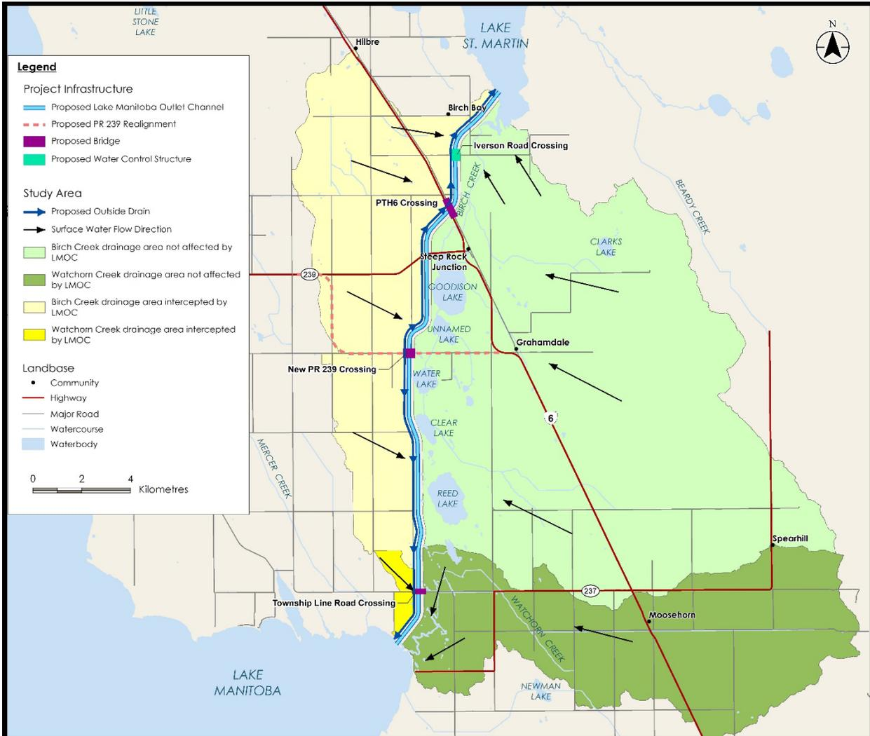
Figure 2: LMO Outside Drain Arrangement
