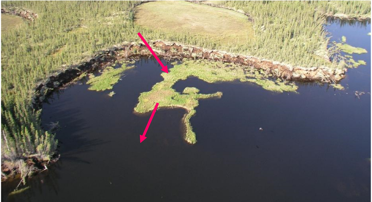
Photo 2-3: Shoreline peatland breakdown in Kettle Generation Project reservoir.
