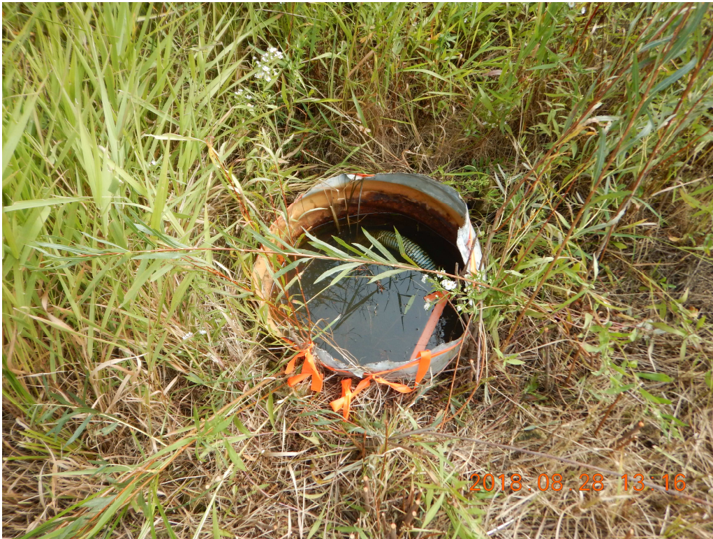
Photo 2: Low level sampling pipe and protective steel casing at 5A1. Cover was missing in during 2018 springs inspections. MI added cap and marker in 2018.
